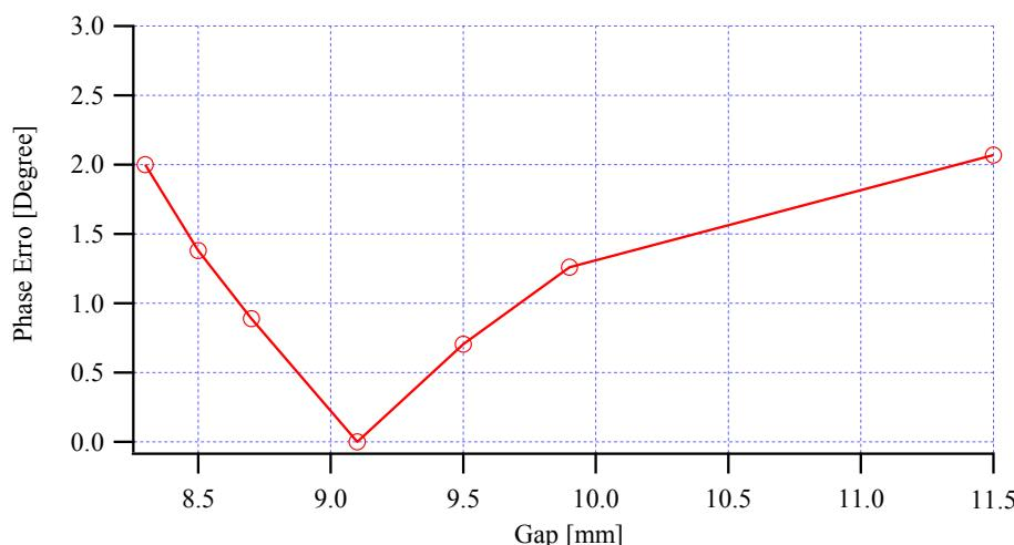
Phase error variation of the ideal undulator due to girder deformation
