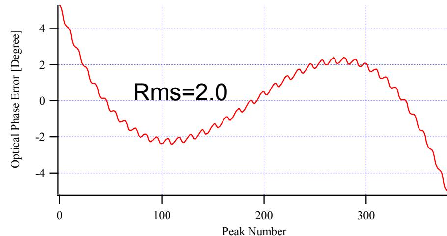
Example of the phase error at min gap due to the girder deformation
