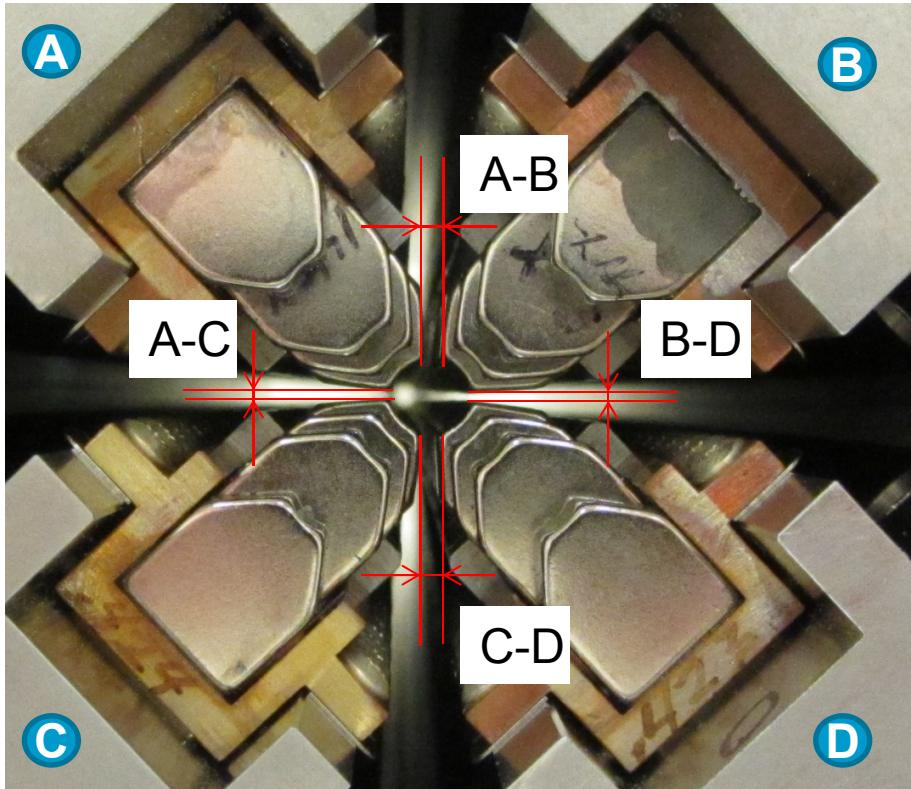
For measurements plastic filler gauge was used. Measurement accuracy ~ 25 µm.
