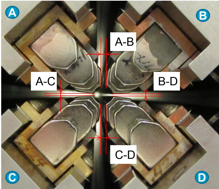
For measurements plastic filler gauge was used. Measurement accuracy  $\sim 25 \mu\text{m}$ . Nominal A-B dimension  $\sim 635 \mu\text{m}$
