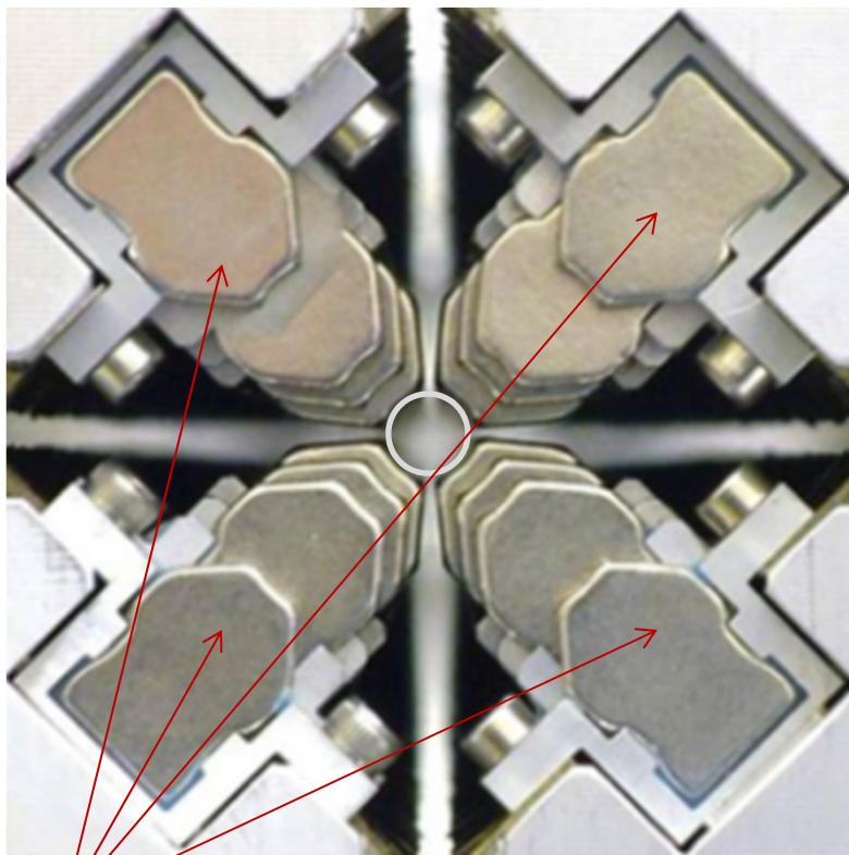
Four independent quadrants of permanent magnets move longitudinally at fixed gap.
