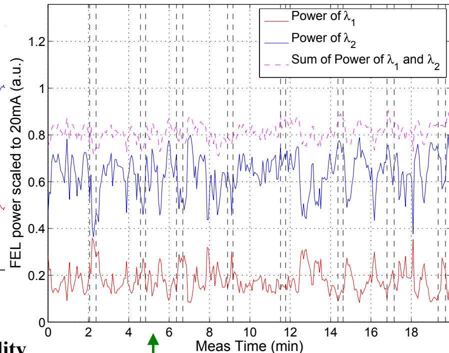
**Degraded Mirrors, poorer temperature stability (Summer):**
