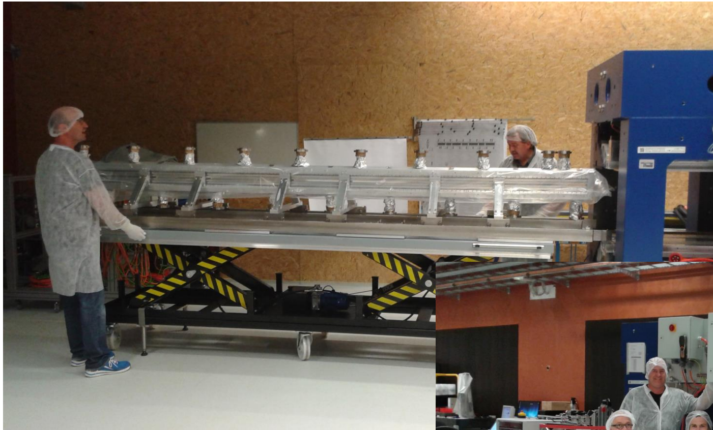
Magnet arrays inserted in the frame
