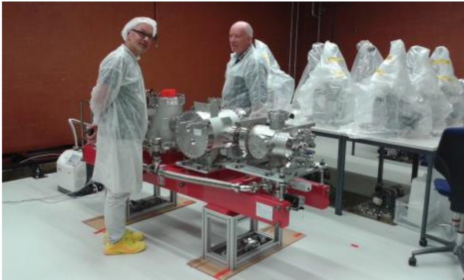
X ray FEL Pulse Energy and Position Monitor at PSI (procured by DESY)
