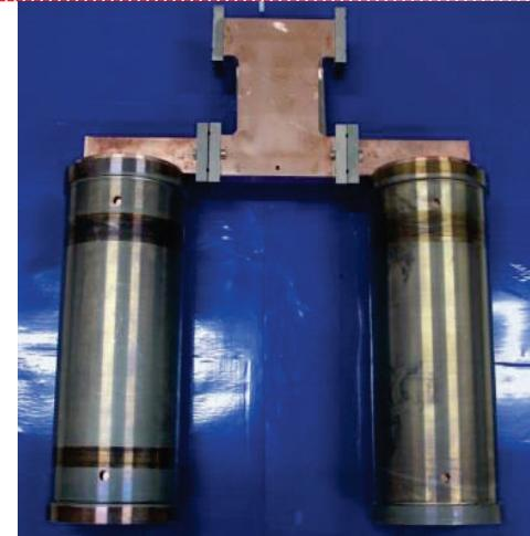
1.8 meters C-band accelerating Structure for SXFEL
