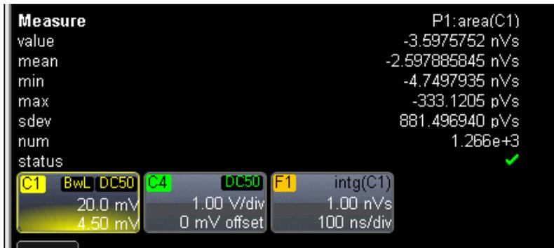
First beam was observed with integrating current transformer during phase scan. The charge was 0.5 nC.
