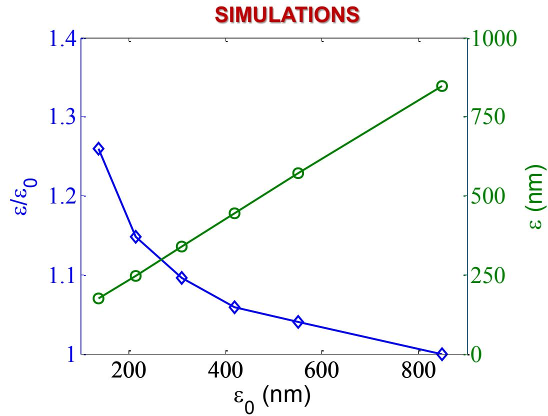
The larger the initial slice emittance, the smaller the relative core emittance blow-up is
