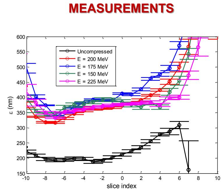
Core emittance increase does not dramatically depend on the beam energy
