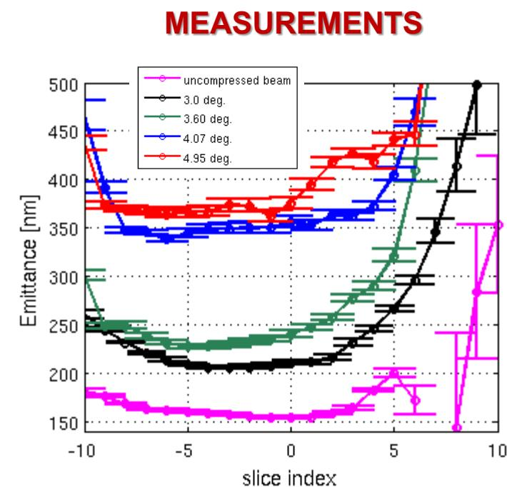
Core emittance increase is smaller for a smaller BC bending angle
