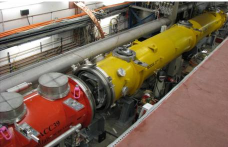
> TESLA type superconducting accelerating modules 1.3 GHz
