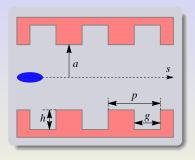
The beam current is  $I_b=20$  A. The frequency  $\omega_0/2\pi$  corresponding to these parameter is 0.3 THz, the gain length is  $L_g=9.9$  cm. The THz FEL would saturate in  $\approx 2$  m.
