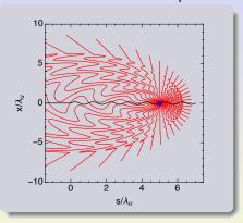
Field lines of the electric field of radiation in undulator. The field propagates ahead of the particle, and generates dynamic wakefield w(s,z). For 1D (helical) undulator:
