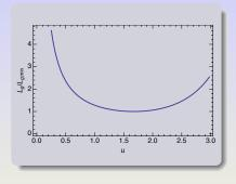
The minimal value is reached at u=1.9 and is equal to 0.74. For the parameter considered above this gives the optimal value of the beam energy:  $\gamma=6.6$  and  $L_g=9.4$  cm. For  $\gamma=10$  the new formula gives  $\ell=11.1$  cm.
