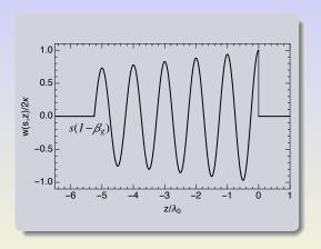
We assume that the damping is weak,  $\mu \ll k_0$ . The sign of the wake is such that the positive wake corresponds to the energy loss, and negative wake means the energy gain. The wake extension (along z) grows with distance s (cooperation length).
