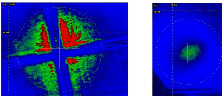
Top: Laser pulses imaged – by help of wire cross - onto the virtual camera (VC2)
