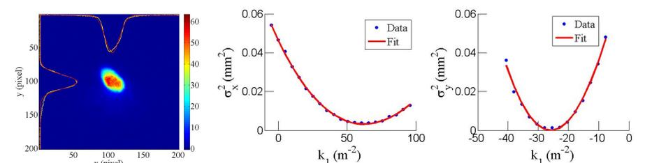
Left: Beam profile observed on phosphor screen when q6 is off.
