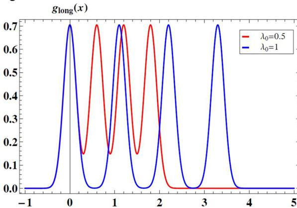
Figure 4: The longitudinal profile of the beam described by Eq. (2) for different parameters  $\lambda_0$ . For all curves  $\sigma'_x = 0.2$ ,  $N_b = 4$ . The values  $x$ ,  $\lambda_0$ ,  $\sigma_x$  have the dimension of length and are measured in identical units.
