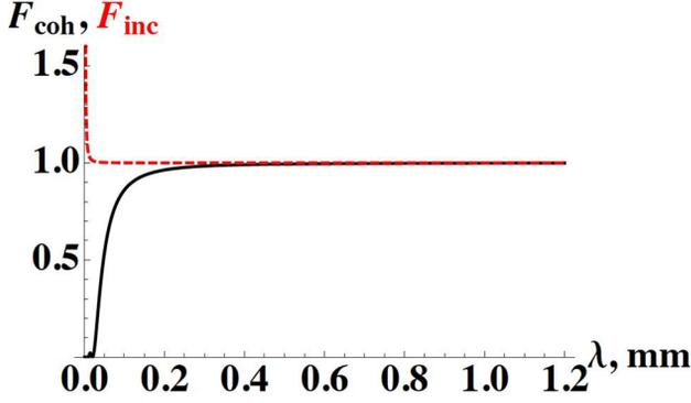
Figure 5: The comparison between  $F_{inc}$  (red dashed curve) and  $F_{coh}^g$  (black solid curve) for the beam of the size  $\sigma_x = 3\mu m$ ,  $\sigma_{y,z} = 14\mu m$ ,  $\lambda_0 = 2\mu m$ ,  $\phi = 0$ ,  $\theta = 30^\circ$ ,  $N_b = 10$ ,  $\gamma = 16$  (energy of LUCX  $E_e = 8MeV$ ).
