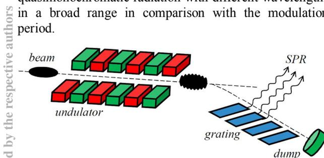
Figure 1: Scheme of using the microbunched beam modulated after passing the undulator for generating intensive Smith-Purcell radiation.
