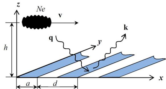
Figure 2: Qualitative scheme of generating the Smith-Purcell radiation.
