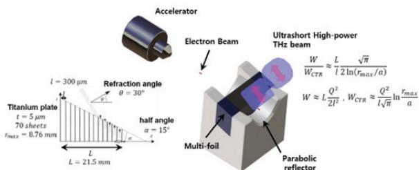
Figure 3: Linear polarization type multifoil radiator.
