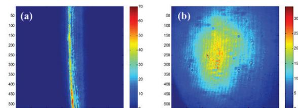
Figure 7: SHB Images of (a) THz generation beam (30 fs) and gate beam (50 fs), (b) Probe beam (300 ps) and gate beam (50 fs).
