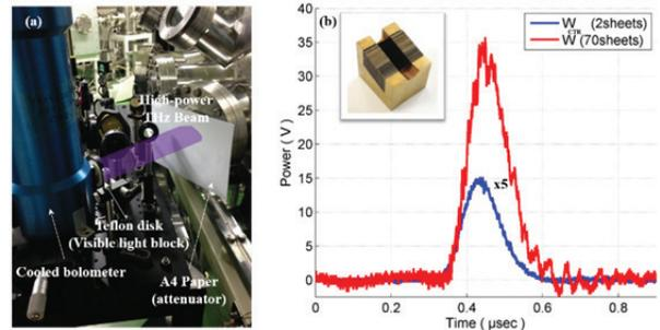
Figure 6: (a) THz power measurement system with cooled bolometer, visible light block and attenuator, (b) Comparison of the power for 2 sheets Ti plate and 70 sheets Ti plates of linear polarization type multifoil radiator.
