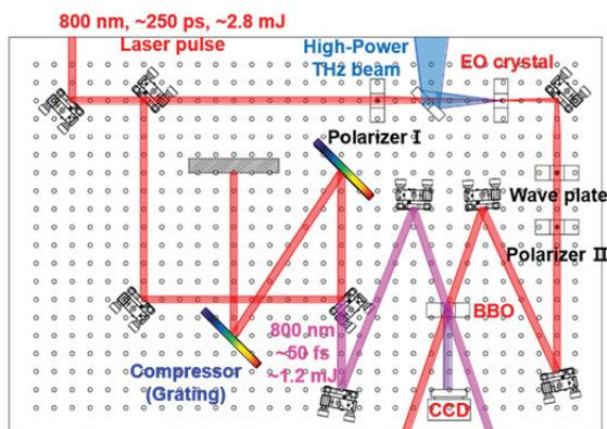
Figure 5: Single pulse measurement system.
