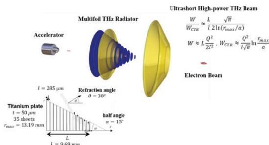
Figure 1: Radial polarization type multifoil radiator.
