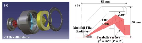
Figure 2. (a) 3D scheme of THz collimator with radiator, (b) The cross-sectional view of THz collimator.
