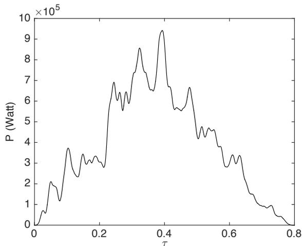
Figure 3: Typical SASE temporal profile with LCLS like parameters at 5 gain length with a non-reflecting boundary and including the advanced field.
