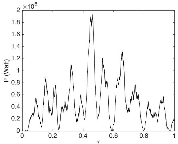
Figure 2: Typical SASE temporal profile with LCLS like parameters at 5 gain length without a non-reflecting boundary.
