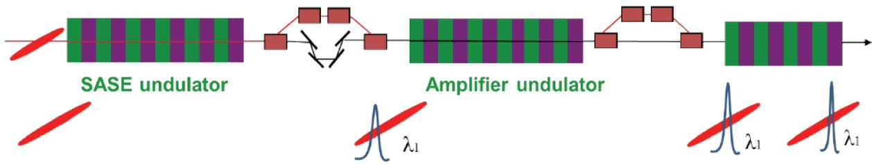
Figure 2: Schematic of the operation mode for soft x-ray self seeding with a chirped electron beam. The second chicane is used as an additional delay to shift the radiation to a “fresh” part of the electron bunch and shorten the pulse duration.
