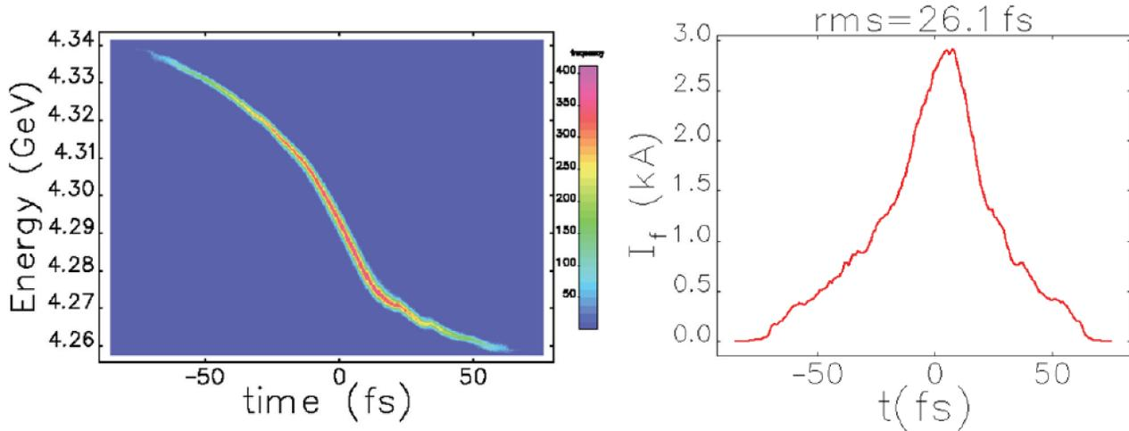
Figure 3: Longitudinal phase space and current profile for the LCLS beam with 150 pC charge and a chirp of 1 % over 30 fs in the core.
