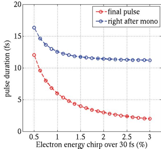
Figure 1: Theoretical expected pulse duration given by Eq. 1 right after the mono and at the end of the undulator. Prediction is in excellent agreement with simulation results for a beam with a 1 % chirp over 30 fs.
