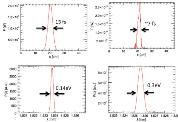
Figure 4: Evolution of the FEL pulse in the time and frequency domain for a chirped beam in the self-seeded operation mode. The left column is after the SXRSS monochromator and the right column is after 20 m of amplification before the second chicane.
