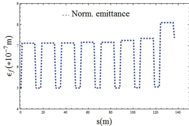
Figure 4: The normalized emittance along the arc. The emittance growth at the end is  $0.24\mu\text{m.rad}$ .
