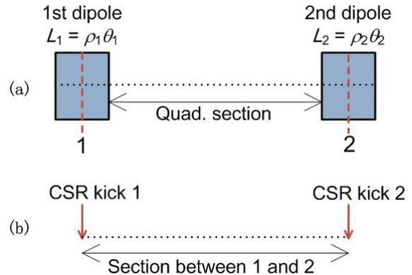
Figure 1: Schematic layout of a two-dipole achromat and physical model for the analysis of the CSR effect with two point kicks. The point 1 and 2 indicate the centres of the first and the second dipole, respectively.
