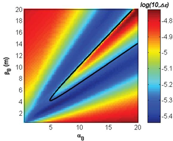
Figure 3: (color online) Numerical simulations of final emittance growth by scanning initial C-S parameters in a symmetric DBA with large compression factor 4.5. The initial transverse emittance is  $1\mu\text{m.rad}$ . Black Line satisfying the CSR-suppression condition Eq. 10.
