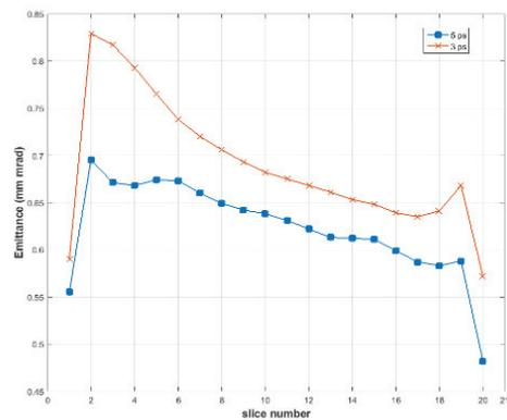
Figure 7: Comparison of optimized slice emittances with laser pulse 3 and 5 ps.
