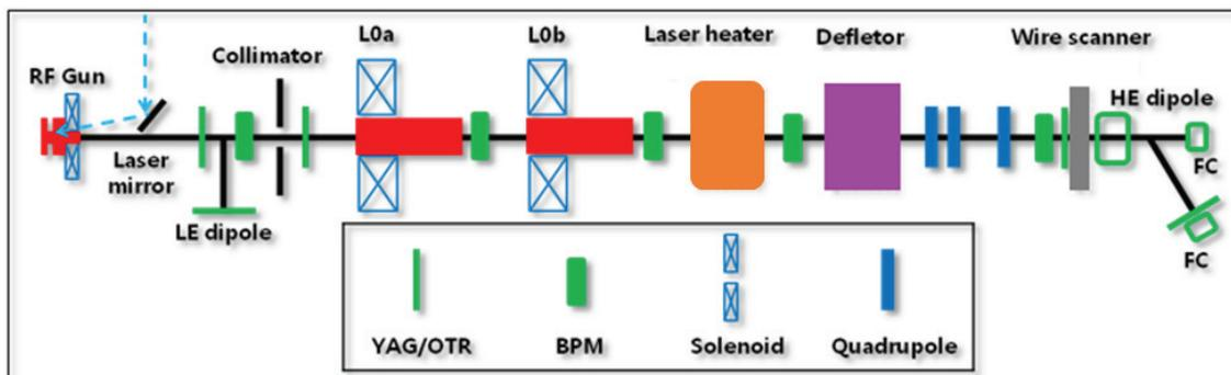
Figure 1: Schematic layout of Injector Test Facility at Pohang Accelerator Laboratory.
