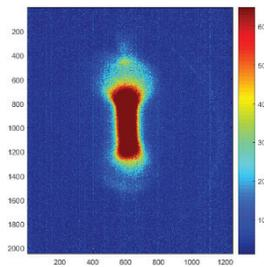
Figure 3: Streaked beam image by the RF deflector on the YAG screen. The head of a bunch is streaked to the top.
