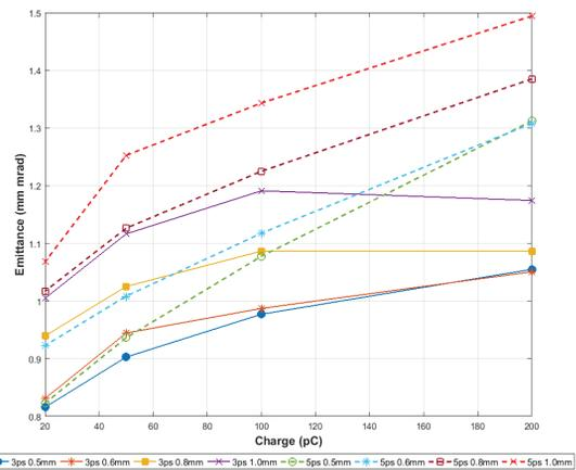
Figure 4: Measured projected emittances at different beam charges, UV laser sizes and pulse lengths. Solid lines describe the UV laser 3ps pulse length and dashed lines describe 5 ps.
