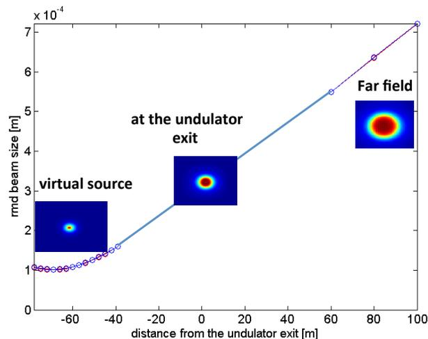
Figure 5: Simulation gives wave front at the exit of the undulator, then it is propagated backward and forward giving the waist (source) and the far field.
