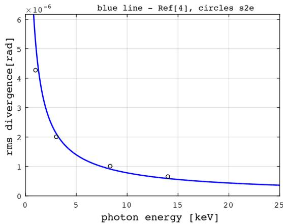
Figure 3: HK Divergence Model (blue line) compared to start-to-end simulations and forward propagation (circles).
