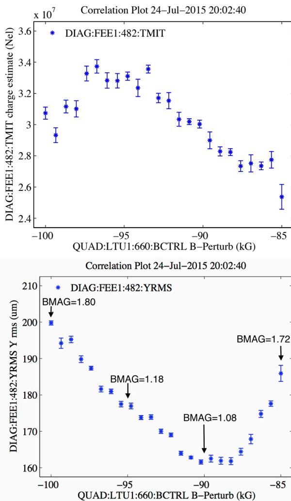
Figure 10: Top plot: x-ray intensity varies with quadrupole scan. Bottom plot: beam divergence changes with match change in the undulator.
