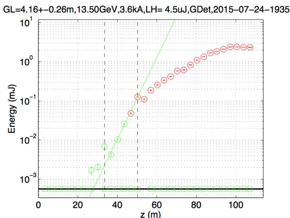
Figure 8: The gain length is measured by a system of gas detector PMTs (photomultiplier tubes) at different high voltage settings to achieve a large dynamic range.
