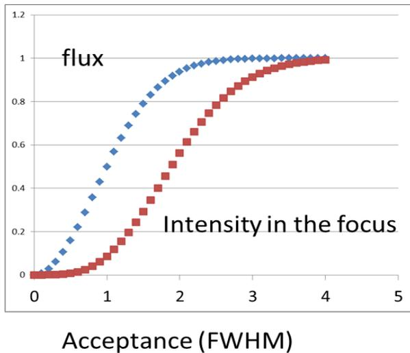
Figure 1: Vertical axis is relative intensity, horizontal axis acceptance of mirror systems cutting in both planes. Blue line is the intensity cut off by mirrors. Red line is the intensity at a downstream focus. Diffraction effects are taken into account.
