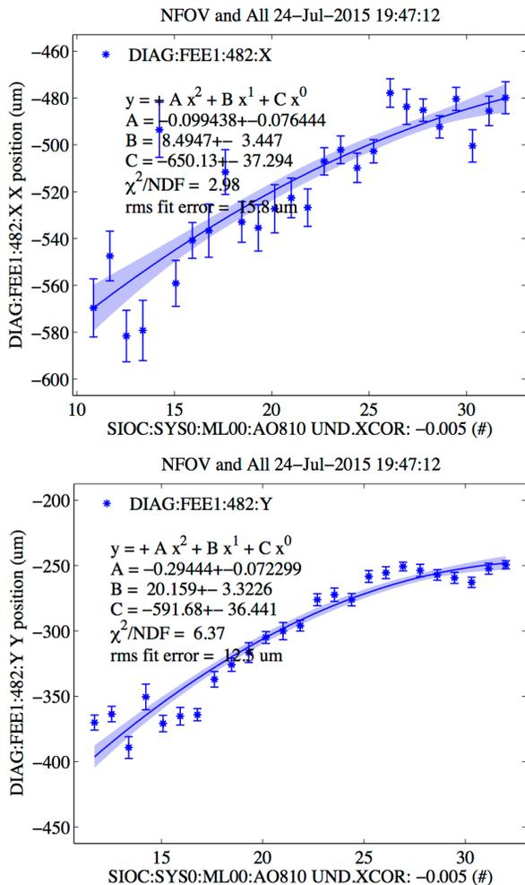
Figure 9: Electron beam is kicked at different points to suppress lasing beyond each point. X-ray position is measured at the imager 87 meters after the undulator.
