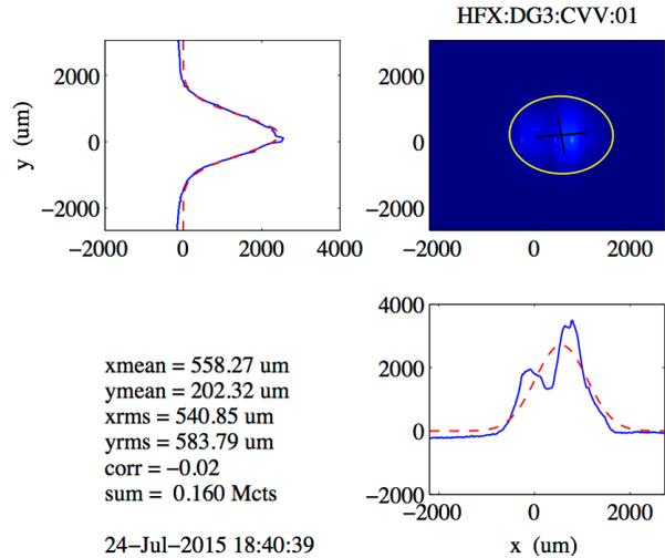
Figure 2: Beam size measured at the Far Hall 335 meters from the end of the undulator. Energy is 8.2 keV. Note the horizontal distortion is due to mirror figure error and diffraction effects [2].
