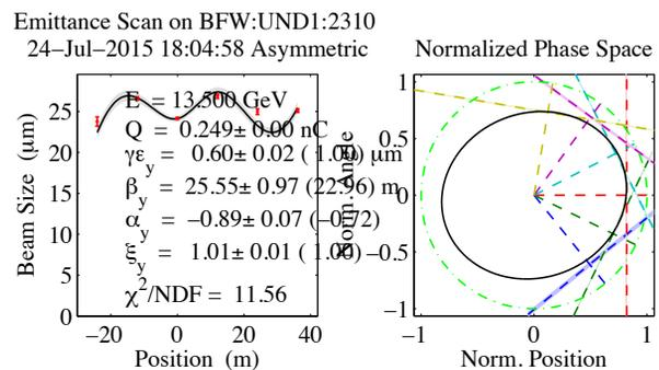
Figure 7: Vertical beta measurement in the undulator using 6 “beam finder wires”. Beta match parameter is 1.01 +/- 0.01 with perfect being 1.0.
