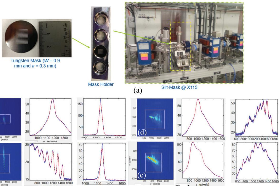
Figure 3: (a) Slit-mask installed in the X115 (BC1). (b) X120-focus with Q115 skew quad (b) OFF and (c) ON at 140 pC per micro-pulse. X124-focus with Q115 skew quad on, (d) 60 pC and (e) optimized.
