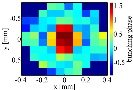
Figure 5: Transversely binned phase of the bunching in the electron bunch. The bunching is given in rad with respect to the center of one slice in GENESIS 1.3 for  $M^2 = 5.0$ .
