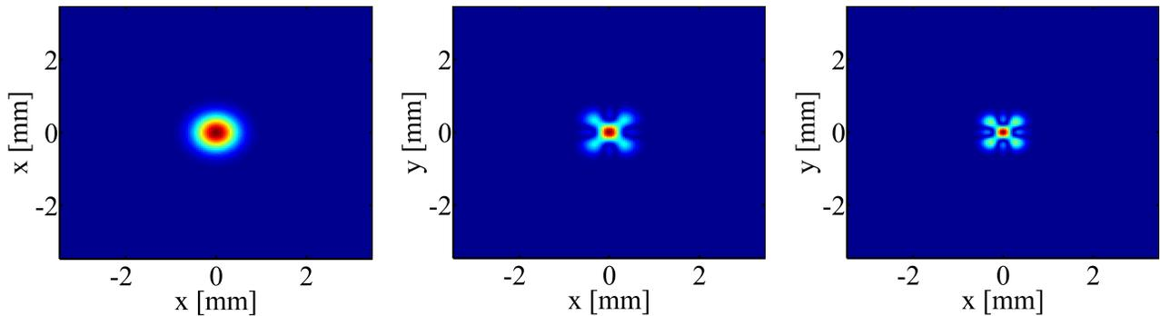
Figure 1: Transverse intensity profile of a laser beam with  $M^2 = 1.0$  (left),  $M^2 = 2.0$  (center) and  $M^2 = 3.0$  (right). The color code shows the relative intensity on a linear scale, where dark red is the are with most intensity and blue is no intensity.
