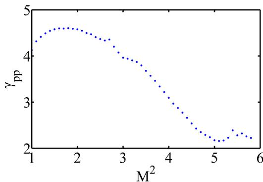
Figure 3: The modulation amplitude  $\gamma_{pp}$  induced by the seed laser as a function of its beam quality factor  $M^2$ .
