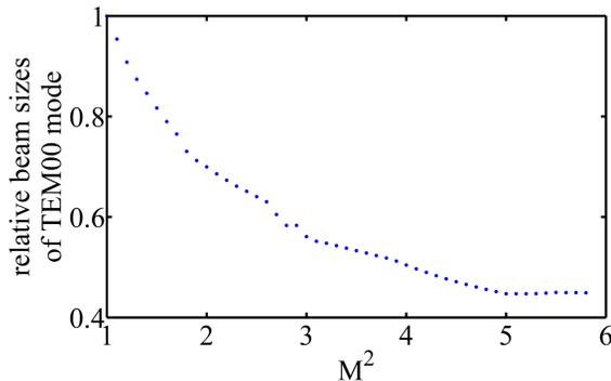
Figure 2: Relative transverse size of the  $TEM_{00}$  mode as a function of its beam quality factor  $M^2$ .
