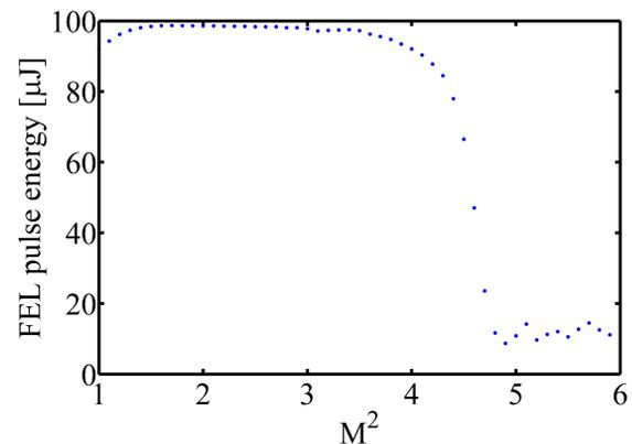
Figure 4: FEL pulse energy after the 4th radiator as a function of its beam quality factor  $M^2$ . The saturation energy increases rapidly between  $M^2 = 4.0$  and  $M^2 = 5.0$  and with this the power after the sFLASH undulators decreases.
