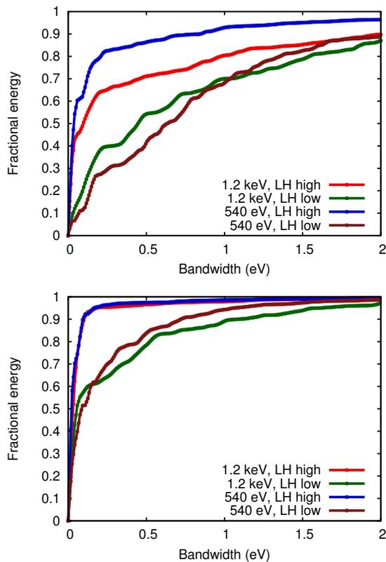
Figure 5: Spectral properties for self-seeding (top) and EEHG (bottom) for various wavelengths and laser heater settings, summarized in terms of the fraction of energy contained with a given bandwidth window.
