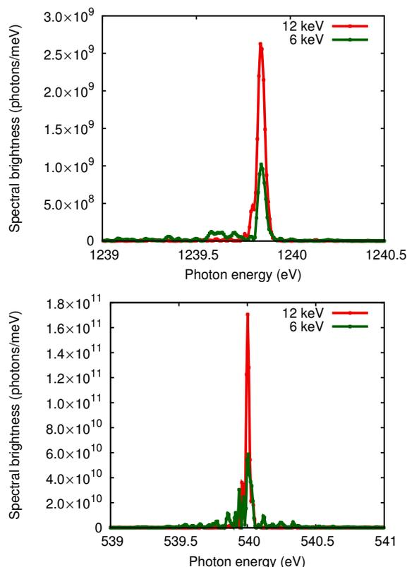
Figure 4: Spectral profiles of the final x-ray pulses for EEHG, at different wavelengths and for different laser heater (LH) settings.
