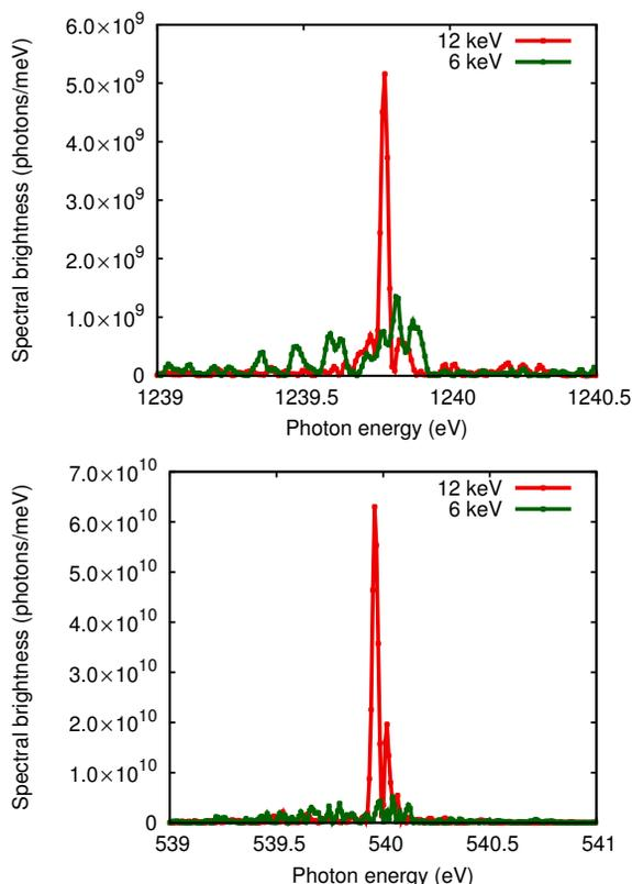
Figure 3: Spectral profiles of the final x-ray pulses for self-seeding, at different wavelengths and for different laser heater (LH) settings.
