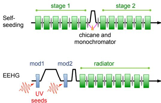
Figure 2: Beamline layouts using self-seeding (top) and EEHG (bottom).
