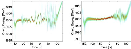
Figure 1: Longitudinal phase space for a 300 pC bunch with the laser heater inducing a 6 keV energy spread (left) and a 12 keV energy spread (right).
