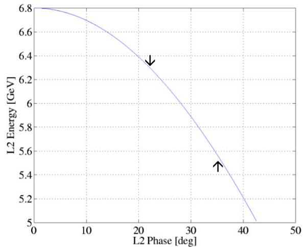
Figure 4: Energy gain due to reduced L2 phase.
