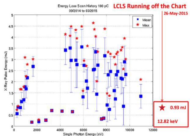
Figure 8: Pulse energy [mJ] versus Photon Energy [eV] shows the 12.8 keV nearly 30% above the typical hard x-ray running conditions.
