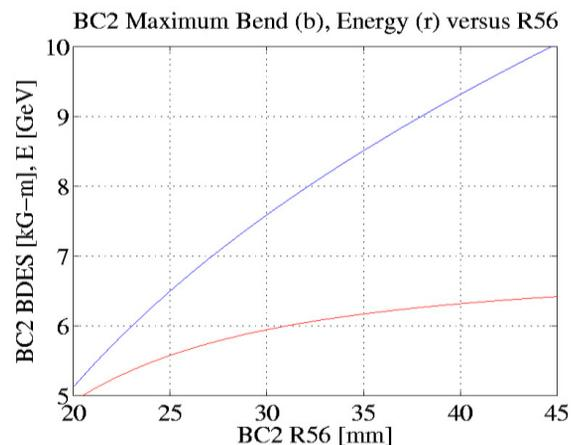
Figure 1: BC2 maximum bend strength and L2 energy versus R56 of the BC2 chicane.
