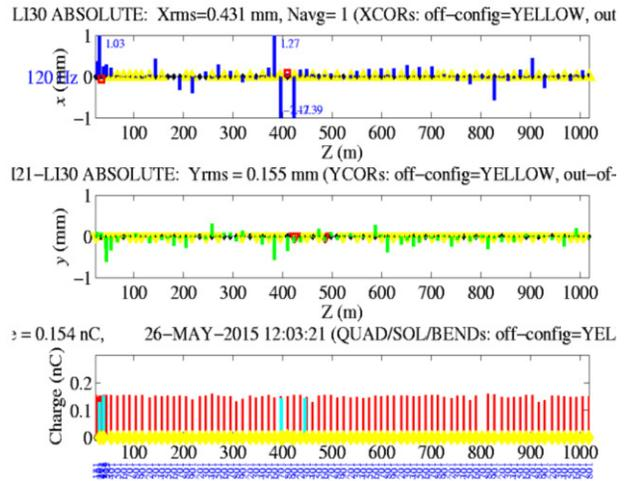
Figure 3: The orbit around BC2 (z = 400 m) had variations of +1.3 mm and -2.4 mm in x, about ten times worse than the rest of the linac.
