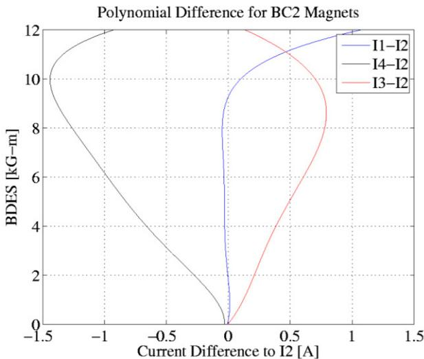
Figure 2: The difference of the bend fields with the respect to the second magnet is plotted versus the required current difference to achieve the same field strength.
