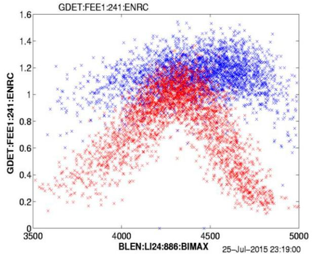
Figure 7: FEL performance via Gas Detector (GDET) [mJ] versus the BC2 peak current [A]. The initial red distribution shows a strong the dependence to peak current, while the tuned up data in blue shows the final performance.
