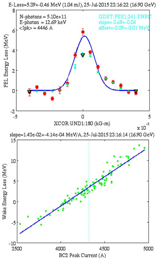
Figure 10: Energy loss scan at 12.8 keV (top) and the calibration measurement with peak current (bottom).
