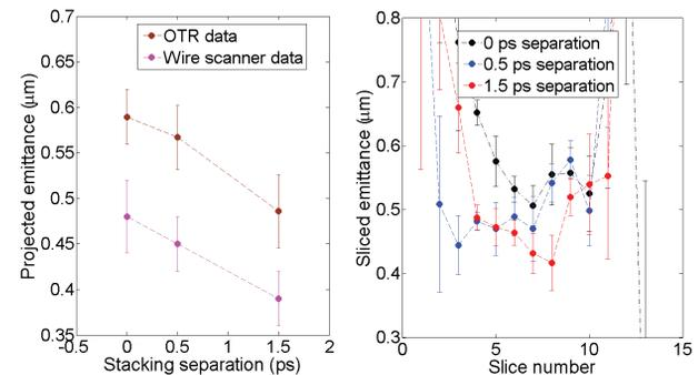
Figure 7: Measured projected (left) and slice (right) emittance (250 pC) with different separation for stacking two  $\sim 1.9$  ps FWHM pulses.
