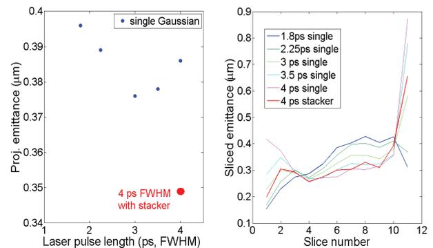
Figure 6: Simulated projected (left) and slice (right) emittance dependence on the single Gaussian laser and a stacked pulse 4 ps FWHM for 180 pC.
