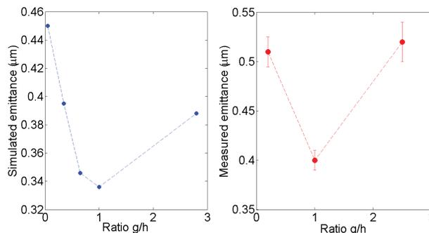
Figure 3: Simulated (left) and measured (right) emittance for different  $g/h$  of lineout intensity ratio for 150 pC.
