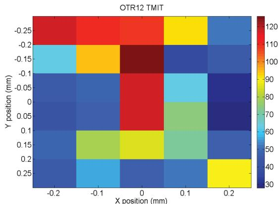
Figure 8: Measured COTR signal in arbitrary units for different laser locations on the same cathode.
