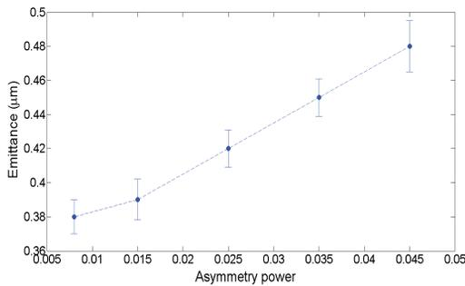
Figure 5: Measured emittance dependence on the asymmetry power for a fixed symmetry power of 0.025.
