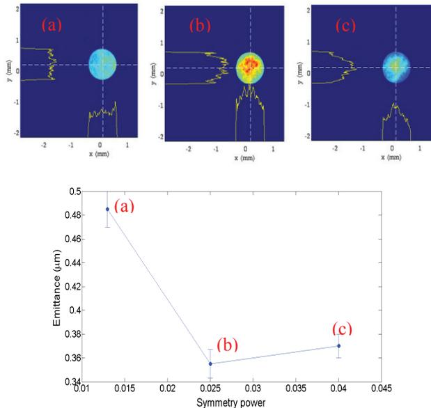
Figure 4: Laser shapes and related symmetry power vs. measured emittance for a fixed asymmetry power  $<0.01$ .
