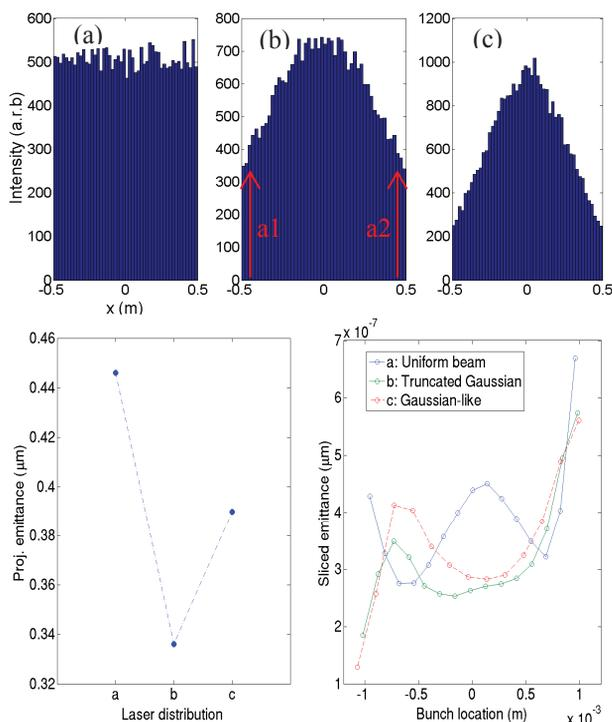
Figure 1: Spatial laser lineout distributions (top), (a), (b) and (c) represent uniform-like, certain truncated-Gaussian and Gaussian-like spatial distributions; corresponding projected (bottom, left) and slice emittances (bottom, right) for 150 pC.
