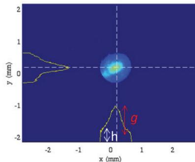
Figure 2: Example of regular smooth beam distribution parameterized by  $g/h$  of the lineout intensity ratio.
