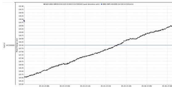
Figure 2: 24 hour RADFET 24 hour dose for 9.5KeV X-rays.
