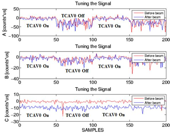
Figure 7: Undulator PMT radiation “Persistence” Scope Integration strip chart with/without TCAV0 Double Pulse Dark Current Suppression.
