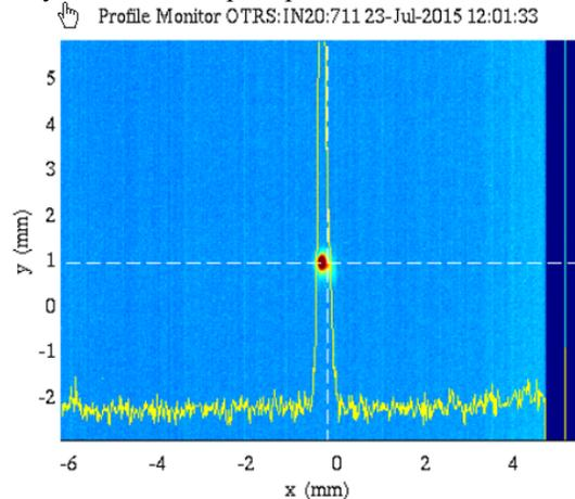
Figure 10: OTR beam image with deflector cavity enabled. Orbit corrected with fine timing of RF drive.
