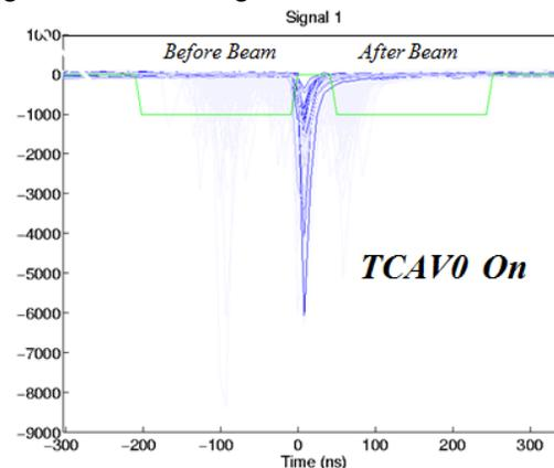
Figure 6: Dark Current Radiation is no longer observed in undulator when the TCAV is enabled with the double pulse.
