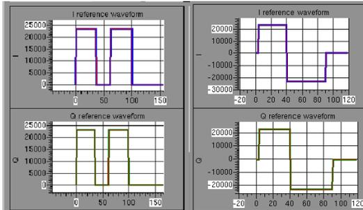
Figure 3: LCLS Control system display of I&Q waveform for dark current sweeper. 3a: RHS:150ns gap. 3b: LHS- "NoGap".
