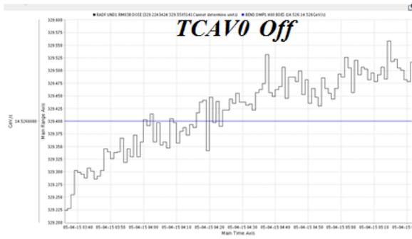
Figure 8: Typical 300mR/hr Radiation dose during 9.5KeV operation.
