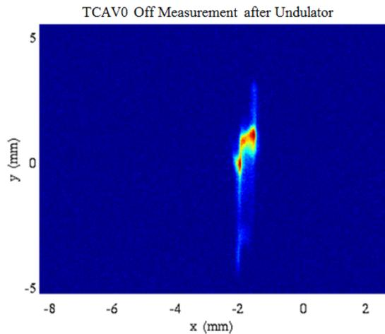
Figure 11: Beam Profile measurement after undulator with Dark Current Sweeper disabled.
