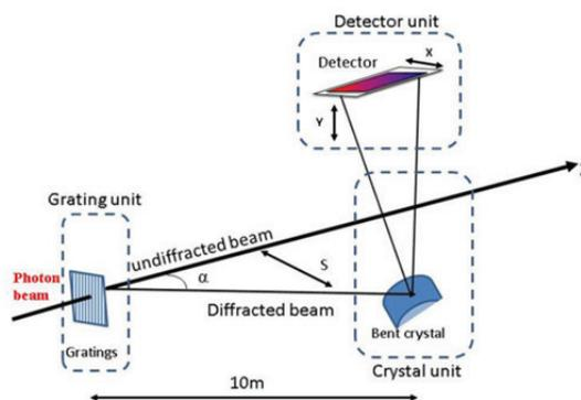
Figure 9: Schematic view of the HiREX setup.
