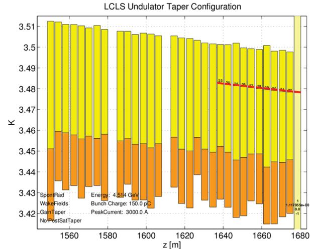
Figure 10:  $K$  values of the LCLS micro-bunching undulators segments for Delta operation in regular afterburner mode.
