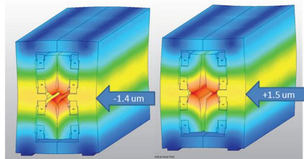
Figure 6: Shape deforming of Delta due to the transverse magnetic forces of  $\pm 15,000 \text{ N}$ , according to finite element modeling.
