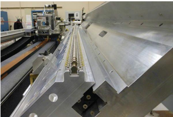
Figure 3: Delta quadrant on the tuning bench.
