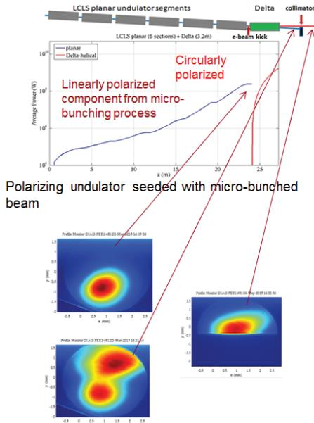
Figure 14: Beam splitting and collimation pushes degree of circular polarization close to 100 %.
