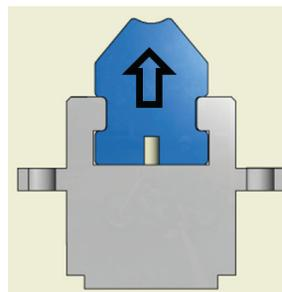
Figure 2: Ni coated PM blocks epoxied to Al holders. (Design by T. Montagne, SLAC)
