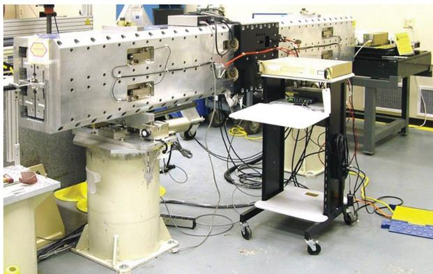
Figure 7: Delta undulator on the field mapping stand.
