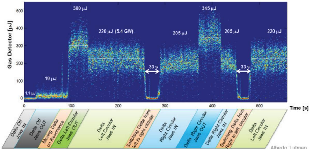
Figure 15: Delta polarization switching during operation.
