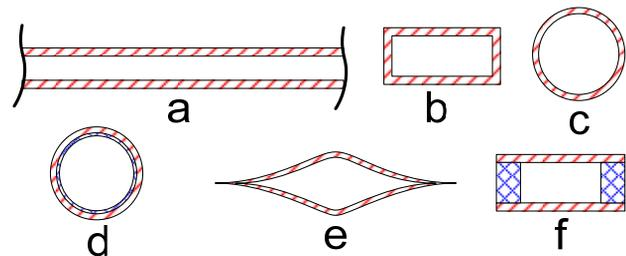
Figure 1: Types of waveguides: a – parallel-plate, b – rectangular, c – circular, d – with dielectric coating, e – special shape, f – rectangular with dielectric walls.
