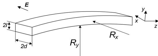
Figure 4: Curvature of a waveguide.
