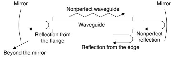
Figure 3: Possible losses in waveguide resonators.
