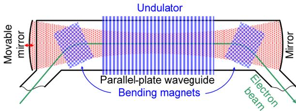
Figure 6: An injection and extraction scheme for a parallel-plate waveguide and adjacent mirrors.
