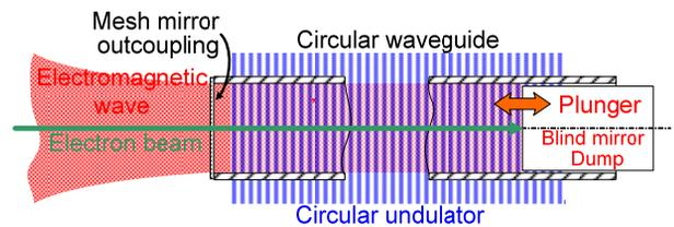
Figure 7: An injection and extraction scheme for a helical geometry and adjacent mirrors.
