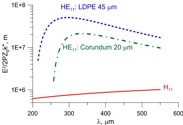
Figure 2: Efficiency of a circular waveguide: all-metal – solid, LDPE coated – dotted, corundum coated – dash-dot.
