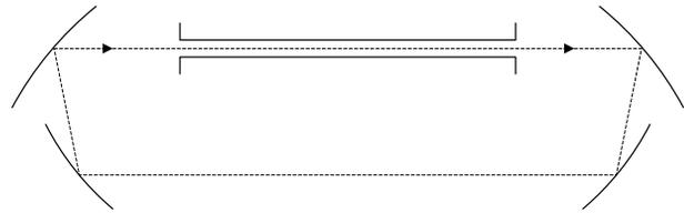
Figure 8: A ring optical resonator.
