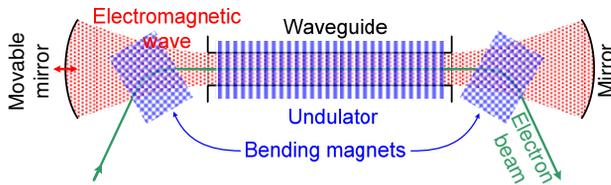
Figure 5: A conventional injection and extraction scheme.
