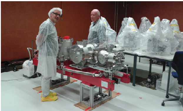
Figure 11: X ray pulse energy and position monitor in the SwissFEL building.
