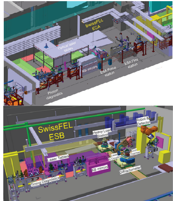
Figure 12: 3D drawings of the End Station A (top) and End station B (bottom).
