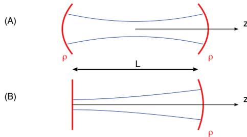
Figure 2: Configuration of resonator.
