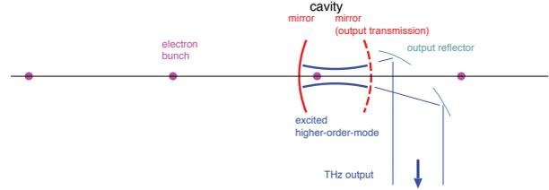
Figure 1: Schematic of resonant CDR.
