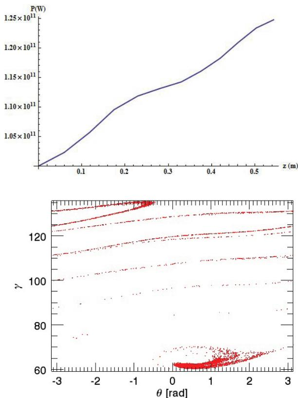
Figure 5: Genesis simulation results showing 25 GW radiation growth and deceleration using 1 kA peak current electron beam.
