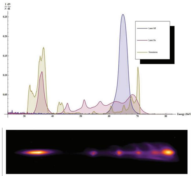
Figure 4: (Above) Deceleration data from Nocibur experiment showing 30% trapping compared with simulation and no laser shot. (Below) Spectrometer image of E-Beam energy spectrum corresponding to the spectra plotted above.
