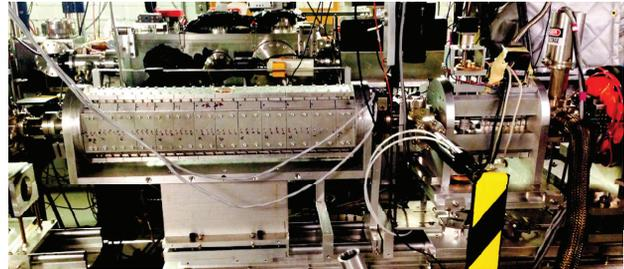
Figure 1: Nocibur undulator and pre-buncher installed in ATF beamline.
