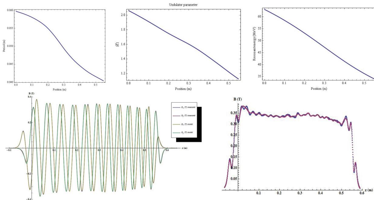
Figure 3: (Top) Design parameters for period tapering, K tapering and resonant energy along undulator. (Bottom) Actual field measurements compared with Radia model field maps.
