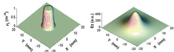
Figure 9: A uniform beam (left) and the LSC electric field (right) in a free space at  $\frac{ka}{\gamma} = 1$ .
