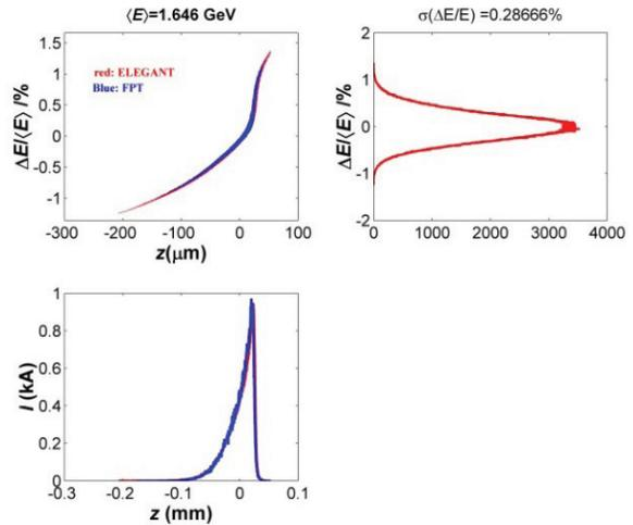
Figure 5: Longitudinal phase space with geometric wake, resistive wall wake and CSR. ELEGANT (red); FPT (blue).
