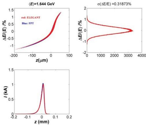
Figure 3: Longitudinal phase space without collective effects. Beam energy at BC2 is 1.644 GeV. ELEGANT (red); FPT (blue).
