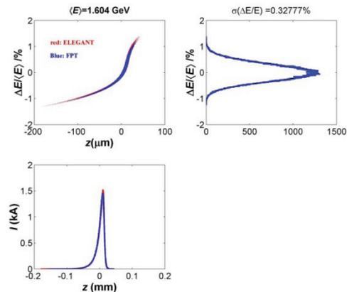
Figure 2: Longitudinal phase space at the end of BC2 without collective effects, beam energy at BC2 is 1.6 GeV. ELEGANT (red); FPT (blue).
