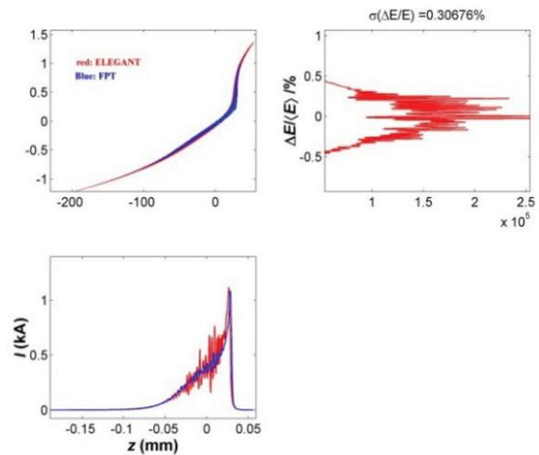
Figure 7: Longitudinal phase space at the end of BC2 with geometric wake, resistive wall wake, CSR and LSC. FPT applies noise reduction trick at L1 and uses 8 million particles, while ELEGANT uses 50 million particles.
