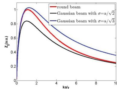
Figure 1: Comparison of the longitudinal space charge impedance of a round uniform and Gaussian beam.
