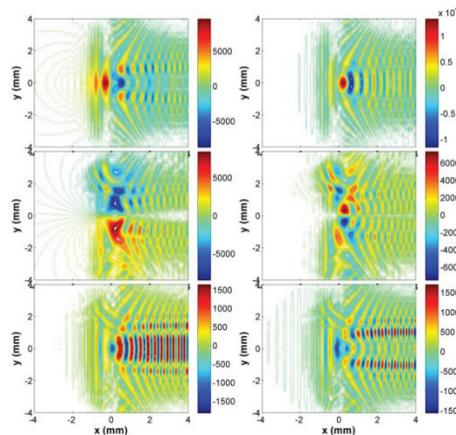
Figure 6: CSR field at the end of last bending magnet for wave number  $k=1.0e6$  [1/m]. The horizontal field (top), vertical field (middle), and longitudinal field (bottom) are shown. Positive x represents outside direction.
