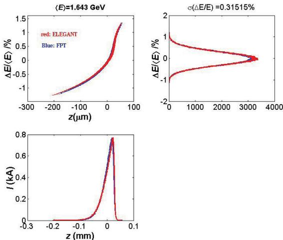
Figure 4: Longitudinal phase space with geometric wake and resistive wall wake effects. ELEGANT (red); FPT (blue).
