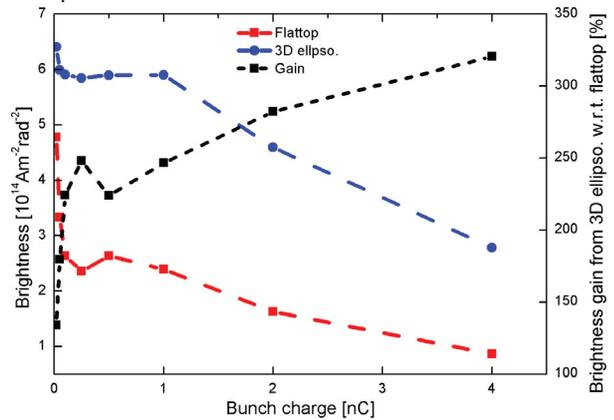
Figure 6: Brightness of the electron beam as a function of bunch charge for flattop and ellipsoidal laser profiles in the left axis, and in the right axis the brightness gain from ellipsoidal beams with respect to flattop ones.
