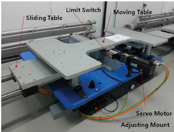
Figure 4: Component of moving support.
