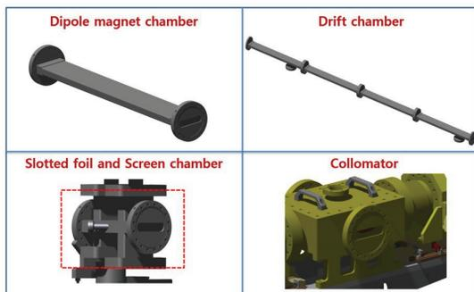
Figure 6: 3D modelling of unified beam chamber.
