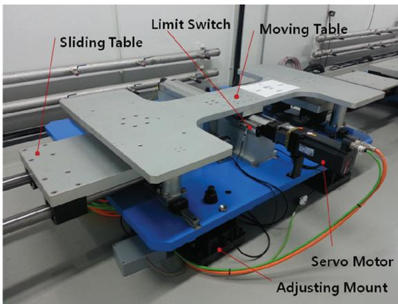
Figure 4: Component of moving support.
