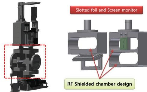
Figure 7: Design of the RF shielded chamber.
