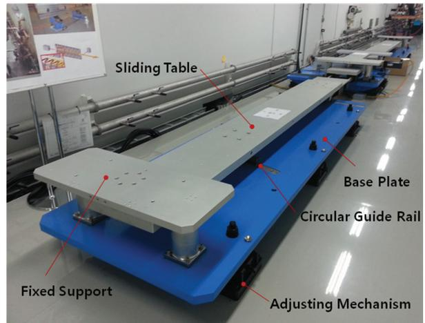
Figure 5: Component of fixed support.
