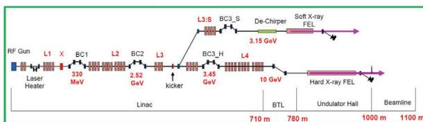
Figure 1: The schematic layout of the 3-BC lattice.
