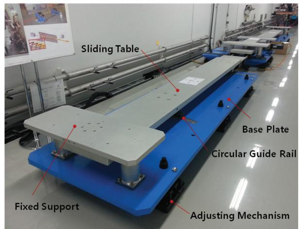
Figure 5: Component of fixed support.
