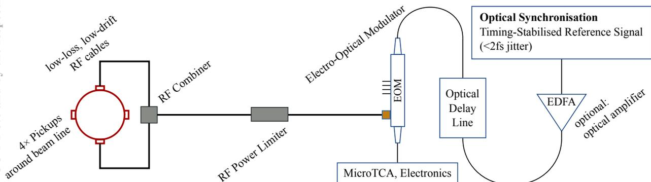
Figure 1: Basic layout of the cabling scheme (only one detection channel is shown).
