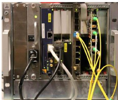
Figure 13: MicroTCA chassis equipped with x2timer, DAMC-FMC25 and DFMC-DSBAM modules.
