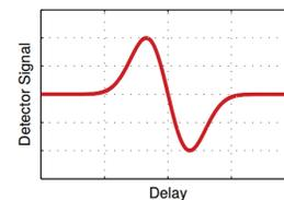
Figure 4: Example signal derived from the balanced optical cross-correlator. Figure source: [13].
