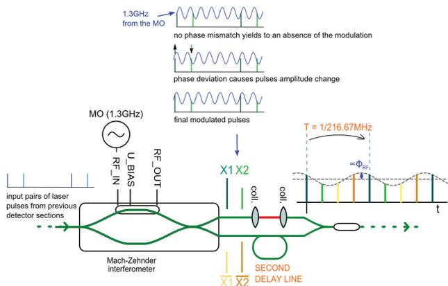
Figure 5: A scheme briefly showing phase detection in an L2RF setup. An output signal containing information about phase mismatch is in case of an MLO of frequency equal 216.67 MHz, which is also a laser pulse repetition rate. Its amplitude is proportional to the phase error.
