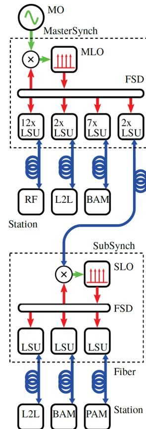
Figure 1: Optical synchronization scheme of the European XFEL. Description of system components: Master Oscillator (MO), Master Laser Oscillator (MLO), Slave Laser Oscillator (SLO), Free-Space Distribution (FSD), Link Stabilization Unit (LSU), Laser-to-Laser synchronization (L2L), Laser-to-RF synchronization (RF), Bunch Arrival-time Monitor (BAM) - beam diagnostics directly using the laser pulse train, Photon Arrival-time Monitor (PAM). Figure source: courtesy of Cezary Sydlo
