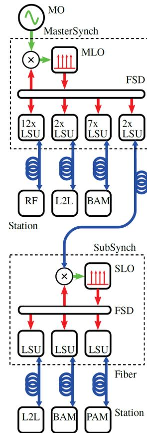
Figure 1: Optical synchronization scheme of the European XFEL. Description of system components: Master Oscillator (MO), Master Laser Oscillator (MLO), Slave Laser Oscillator (SLO), Free-Space Distribution (FSD), Link Stabilization Unit (LSU), Laser-to-Laser synchronization (L2L), Laser-to-RF synchronization (RF), Bunch Arrival-time Monitor (BAM) - beam diagnostics directly using the laser pulse train, Photon Arrival-time Monitor (PAM). Figure source: courtesy of Cezary Sydlo
