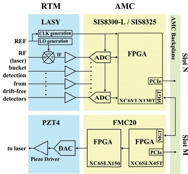
Figure 2: MTCA.4 components for laser locking application. Description of the terms: RTM-Rear Transition Module, a board connected to a specific AMC from the rear side of a MTCA.4 crate, AMC-Advanced Mezzanine Card, LASY-LAser SYNchronization board, SIS8300-L/SIS8325-digitizer board, where the controller is implemented, PZT4-4 channel piezo driver to control the piezo of the laser, FMC20-dual FPGA mezzanine card, here used for backplane and RTM interconnections.
