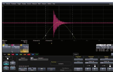
Figure 4: Raw signal of cavity BPM pick-up y-direction port. This output signal was down converted as 200 MHz and measured by using oscilloscope.
