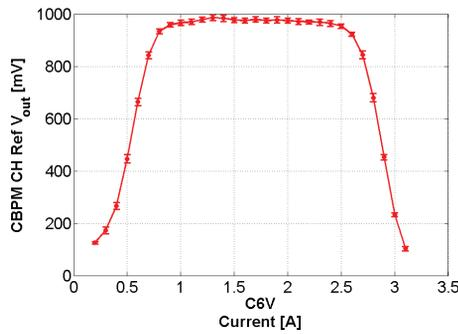
Figure 5: Reference cavity output voltage response to corrector C6V.
