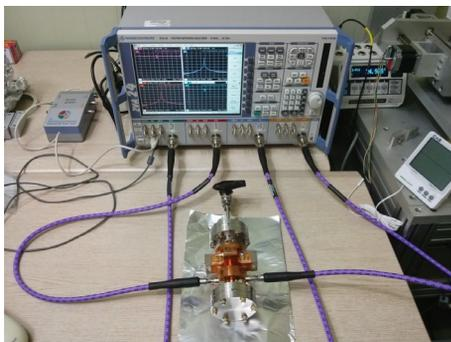
Figure 2: Fabricated prototype cavity BPM pick-up.
