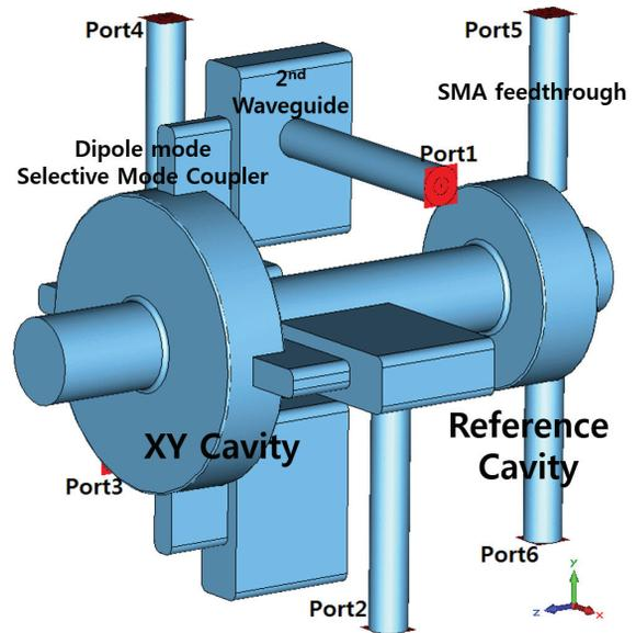
Figure 1: Modeling of PAL-XFEL cavity BPM pick-up vacuum part.
