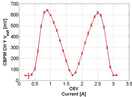
Figure 6: XY cavity y-direction output voltage response to corrector C6V.
