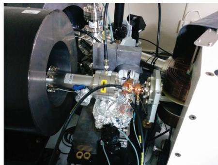
Figure 3: Installed prototype cavity BPM pick-up at ITF dump section.
