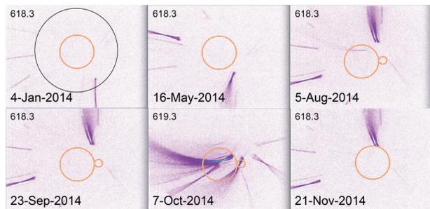
Figure 3: Darkcurrent of the RF-gun with cathode 618.3 and 619.3 measured with a Ce:YAG powder screen during operation in 2014. The red circle indicates the position of the Cs<sub>2</sub>Te film, the black circle the rim of the cathode. The streaks are due to the solenoid field. Pictures were taken under normal operating conditions of the gun (see text).
