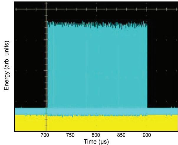
Figure 5: Oscilloscope trace of the laser pulse train used in this experiment. The spacing of the individual pulses is 1  $\mu$ s (1 MHz), the train length is variable, in this example 200  $\mu$ s. The wavelength is 262 nm. The laser pulse energy is measured with a UV sensitive photodiode.
