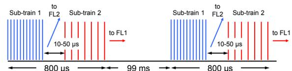
Figure 4: Bunch train sharing between FLASH1 (FL1) and FLASH2 (FL2): one RF pulse (10 Hz repetition rate) is shared by two sub-bunch trains. One train goes to FLASH1, the other is kicked to FLASH2. The sub-trains may have different bunch pattern or charge.
