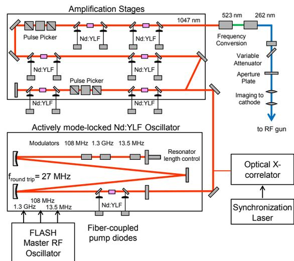
Figure 1: Schematic overview of laser 2 [14]. The oscillator and amplifiers are pulsed with 10 Hz, pulses are a few milliseconds long. The laser 1 amplification stages are very similar. Laser 1 has a shorter oscillator operating at 108 MHz using a 54 MHz AOM and a 1.3 GHz EOM.
