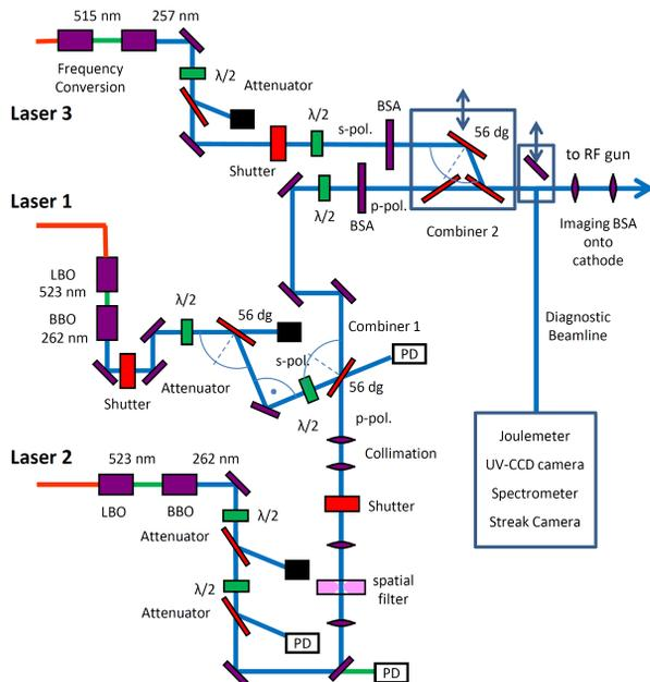
Figure 3: Beamline to combine all three laser systems. See explanations in the text.
