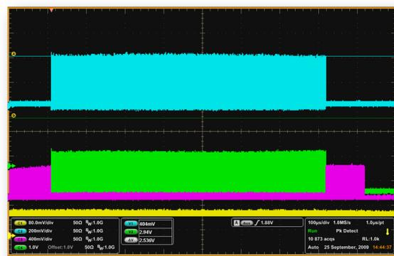
Figure 2: Example of a train of laser pulses [14]. The oscilloscope traces show the pulse train of the 27 MHz oscillator (yellow trace), after preamplification (3 MHz, wavelength 1047 nm, magenta), after conversion to 523 nm (3 MHz, 523 nm, green), and after conversion to the UV (3 MHz, 262 nm, blue). The time scale is 100  $\mu$ s per division. Neither the 27 MHz nor the 3 MHz pulse structure is not resolved. Usually the laser is operated in the 1 MHz mode.
