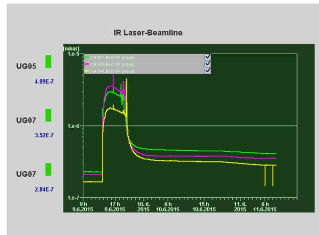
Figure 2: Pressure rise in laser transport vacuum system due to motors outgassing.
