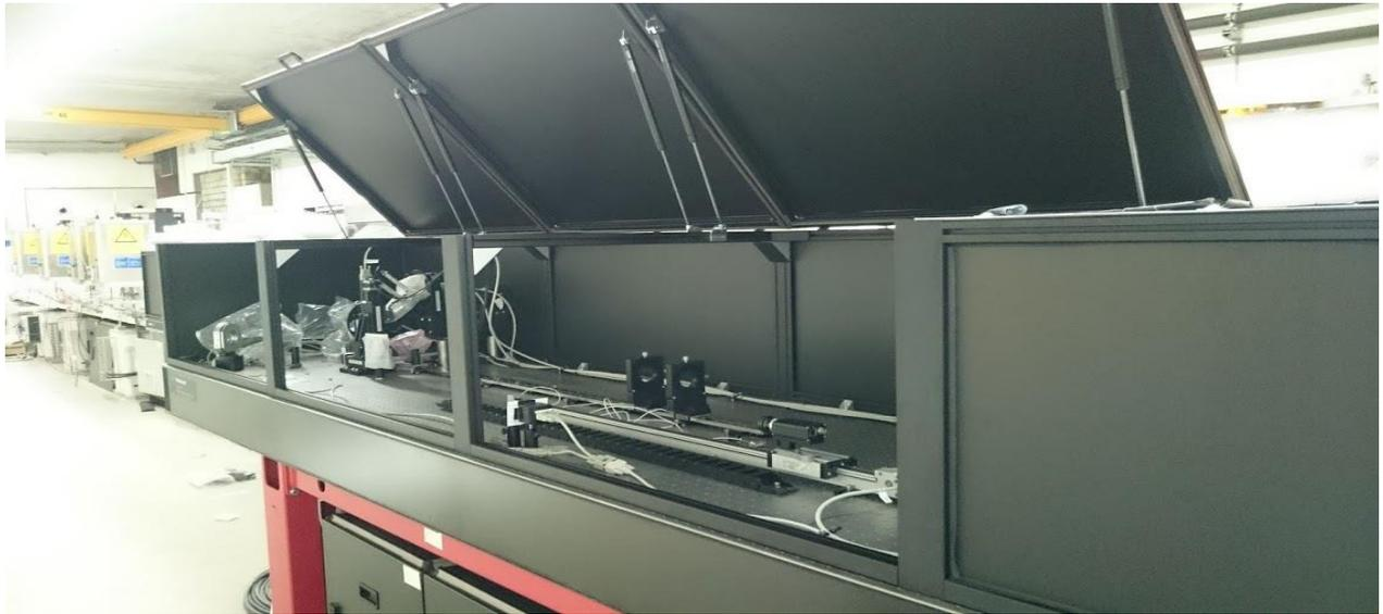
Figure 6: The OS0 when looking downstream. The telescope lenses are clearly visible in the center of the optical table. More optical components toward the end of the table are at the time covered with plastic bags for dust protection.
