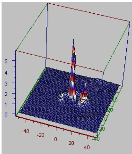
Figure 4: The 3D image shows that the signal is strongest when the laser is hitting the center of the mirror. The bottom plane is the scan area whereas the height represents signal intensity, units are arbitrary.
