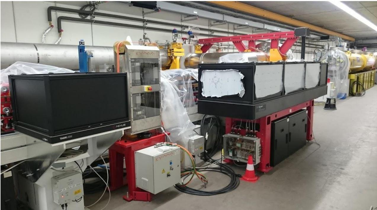
Figure 3: Overview over the laser heater on LVL7 (injector). The large optical table (OS0) is to the right side, undulator in the middle and the small table (OS1) on the left side. On top of OS0 the horizontal beam contains part of the laser vacuum system which continues along the wall to the right.
