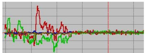
Figure 5: Signal from PSD located at the same distance as the undulator center (arbitrary units). Horizontal-axis is time (~10 s), vertical-axis is position (red is x-position, green y-position). The stabilisation system is turned on after half the time and the position is stabilised significantly.
