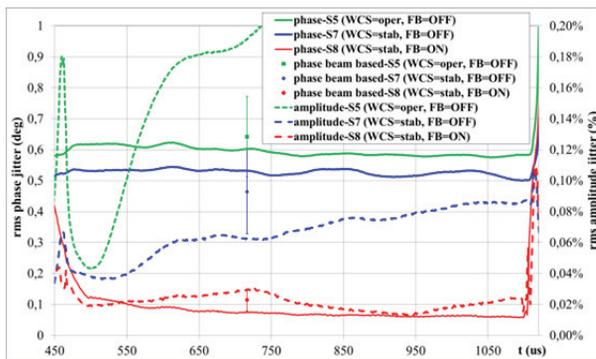
Figure 5: RF gun stability measurements. The RMS phase and amplitude jitter is plotted at left and right axis correspondingly for two regimes of the WCS and deactivated/activated LLRF feedback (measurements S5, S7 and S8). Results of the correspondent beam-based measurements are shown with markers. The horizontal position of these points corresponds to the time of the first electron bunch within the RF pulse.
