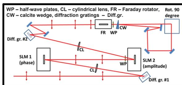
Figure 1: Schematic overview of the 3D shaper.
