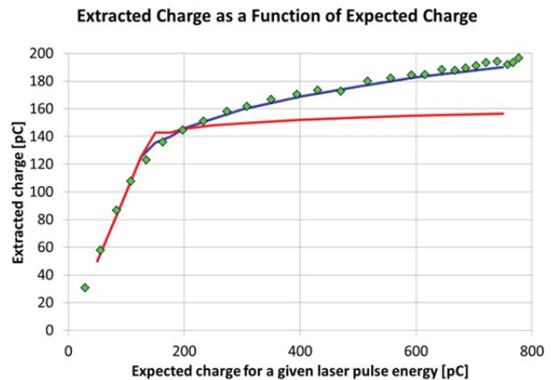
Figure 9: Extracted charge and expected charge given by simulation of a homogenous, transversely flat-top laser pulse (red) and the same distribution with a photonic halo (blue), and measurement of charge actually extracted (green).
