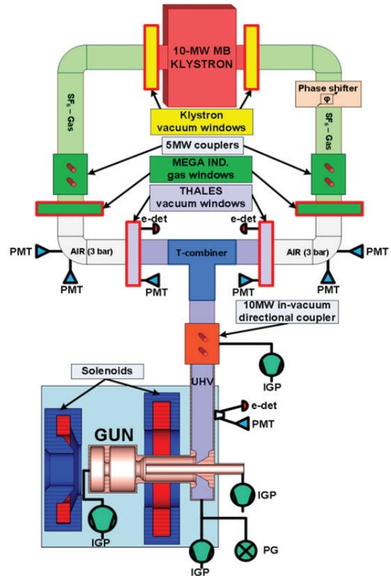
Figure 4: New gun interlock and RF distribution scheme.
