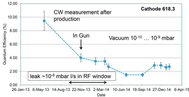
Figure 7: Quantum Efficiency of FLASH's Cs<sub>2</sub>Te Cathode 618.3 during 2013/2014.
