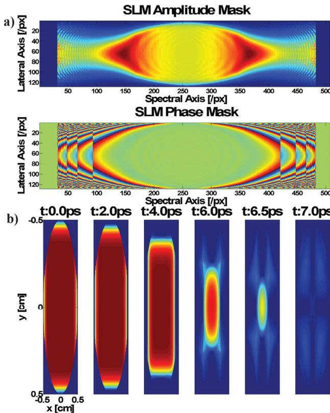
Figure 2: a) The corresponding normalized amplitude and phase masks. b) Temporal slices of a simulated quasi-ellipsoidal laser pulse.  $t=0$  ps corresponds to the temporal center of the laser pulse.
