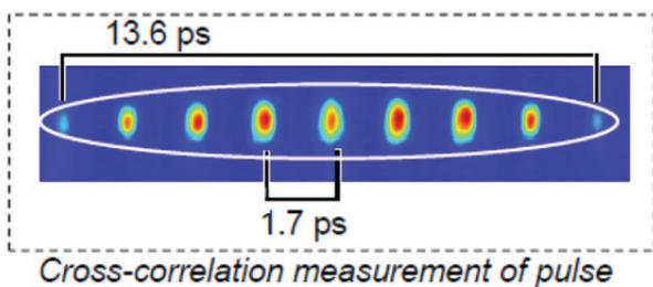
Figure 3: Cross-correlation measurement of a shaped pulse produced in the lab. Shown are  $\sim 250$  fs time slices of the transverse distributions of the shaped laser pulse taken at 1.7 ps intervals throughout the entire pulse duration of 13.6 ps.
