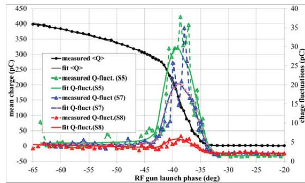
Figure 6: Beam based measurements of the RF gun stability. Measured mean charge and its analytical fit are plotted at the left axis. Charge fluctuations together with fits for three cases of WCS and FB (measurements S5, S7 and S8) are plotted at right axis.
