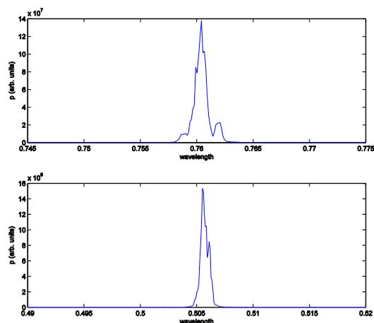
Figure 4: 2nd (a) and 3rd (b) harmonic FEL spectrum at the radiator exit.
