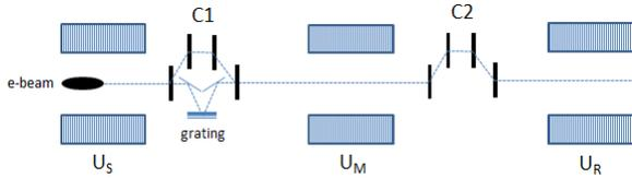
Figure 1: Schematic of HGHG based on self-seeding.  $U_S$  is a SASE undulator resonated at 1.52nm.  $U_M$  is a modulator resonated at 1.52 nm while  $U_R$  is a radiator resonated at 0.76 nm or 0.507 nm. C1 and C2 are chicanes with different values of  $R_{56}$ .
