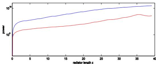
Figure 3: The 2<sup>nd</sup> (blue line) and 3<sup>rd</sup> (red line) harmonic power evolution along the radiator undulators (Different  $A_u$  values.)
