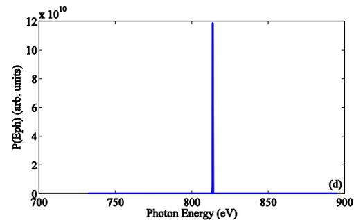
Figure 2: The FEL power at monochromatic SASE stage in time and frequency domain.(a) temporal profile at the exit of  $U_s$ ; (b) spectrum at the exit of  $U_s$ ; (c) temporal profile at the exit of monochromator; (d) spectrum at the exit of monochromator.
