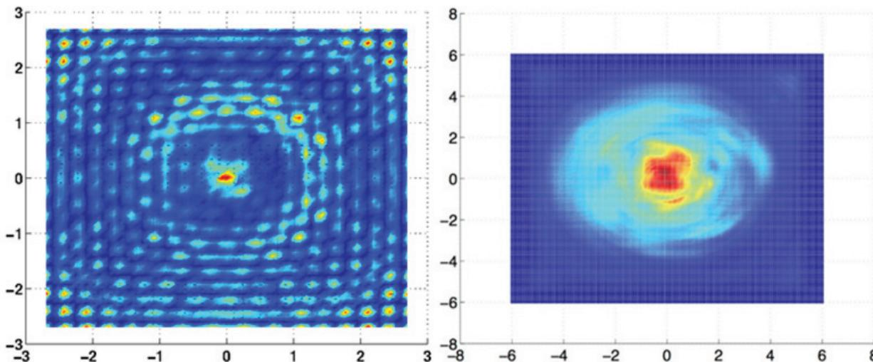
Figure 2: Diffraction before (left) and after (right) the implementation of the absorbing boundary conditions, for identical parameters.
