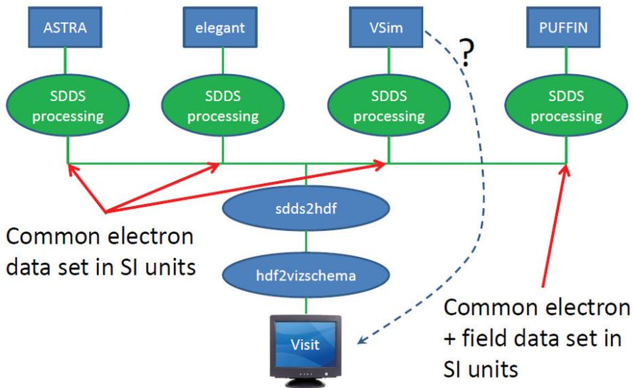
Figure 4: Schematic of the proposed, idealised visualization chain for the simulation suite. SDDS is used for post-processing and VisIt is used for viewing the results after conversion to HDF5 format. Note that VisIt can already directly visualize VSim data, so it may be more convenient to utilize this functionality within this project.
