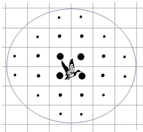
Figure 3: The ‘shotgun’ model of particle spreading. The heavier macroparticle from the coarse accelerator distribution is the shotgun cartridge and the finer shot (of varying size) are the microparticle. The pellets from the shotgun cartridge spread out over the blast radius according to a spreading factor.
