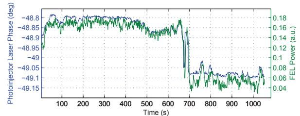
Figure 2: Observed correlation between photoinjector laser phase and FEL output power, prior to introduction of feedback.
