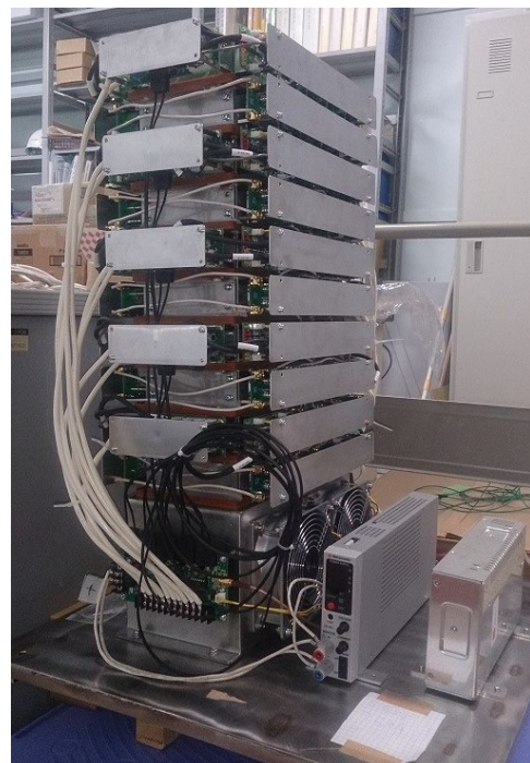
Figure 1: Solid state switch 2nd model for the klystron modulator. The maximum holding voltage is 25 kV and the peak current is 6 kA for 8 \mu\text{s} pulses at a repetition frequency of 60 Hz.
