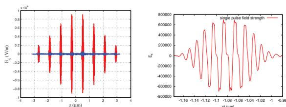
Figure 3: Electrical field strength distribution of the scattering radiation.
