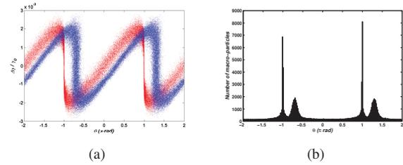
Figure 2: Longitudinal phase space after dispersion section. PEHG in red and HGHG in blue for comparison. 2(a): Longitudinal phase space; 2(b): Particle distribution.
