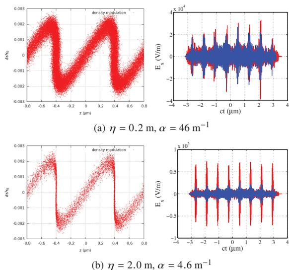
Figure 5: 3-D simulation with the transverse emittance  $\epsilon_x = 1\text{mm-mrad}$
