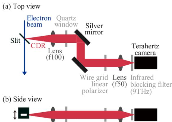
Figure 1: Schematic illustration of the spatial distribution measurement of CDR using a terahertz camera.
