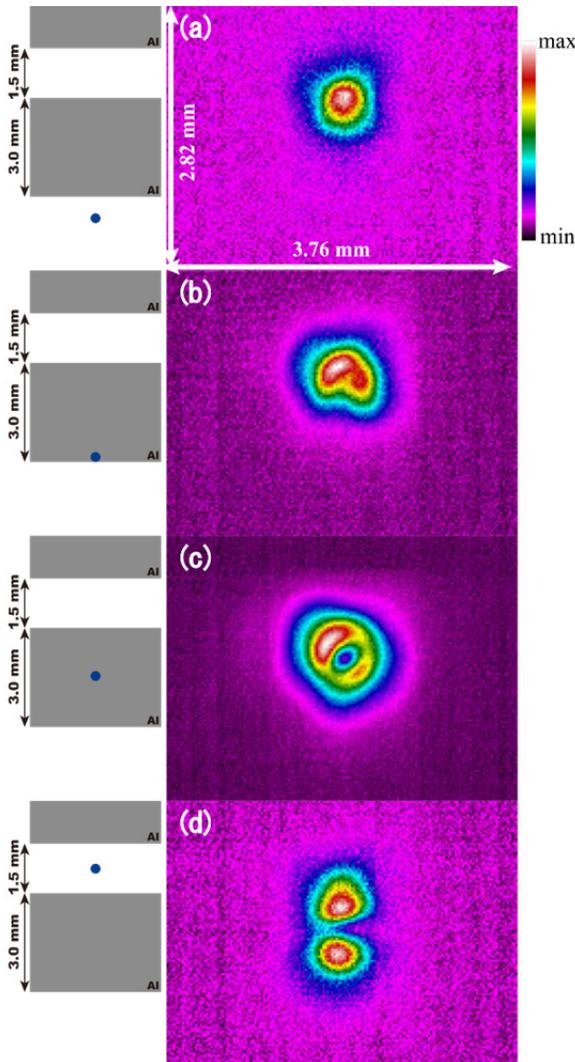
Figure 3: Spatial distribution of the CDR and CTR measured with the terahertz camera. (a) CDR: The electron beam passed in vacuum where 0.7 mm away from the edge. (b) CDR+CTR: The electron beam passed through the aluminium where 0.2 mm inside from the edge. (c) CTR: The electron beam passed through the central of the semi-plane. (d) CDR: The electron beam passed through the central of the rectangular slit.
