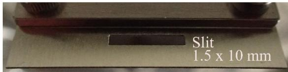
Figure 2: Picture of the rectangular slit target with the dimension of 1.5 mm x 10 mm and edge for generating the CDR.
