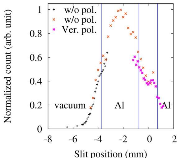
Figure 4: Normalized total counts in area the CDR is detected. The plus and cross symbols are the normalized counts when the polarizer was not used. The square symbol is the normalized counts of the vertically polarized component.
