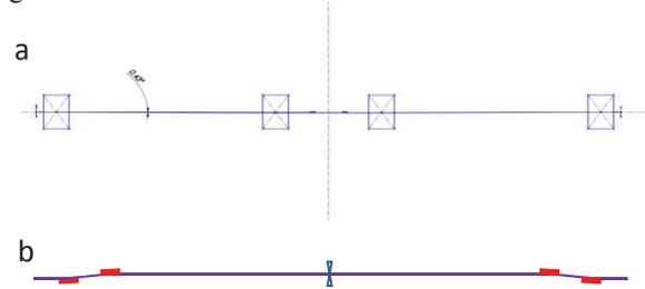
Figure 2: a) The four-dipole bypass chicane with the 4BCM in between the two middle dipoles; b) expanded view of the 4BCM showing the four Si(111) crystals in red and the slit in blue. The total length of the bypass chicane (2a) is 8.63 m whereas the length of the 4BCM (2b) is 0.4 m.
