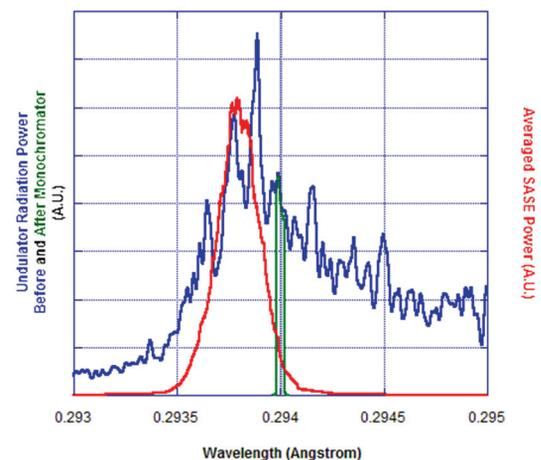
Figure 3: The undulator radiation spectrum before (blue) and after (green) the 4BCM, and the average SASE signal in the exponential gain regime (red).
