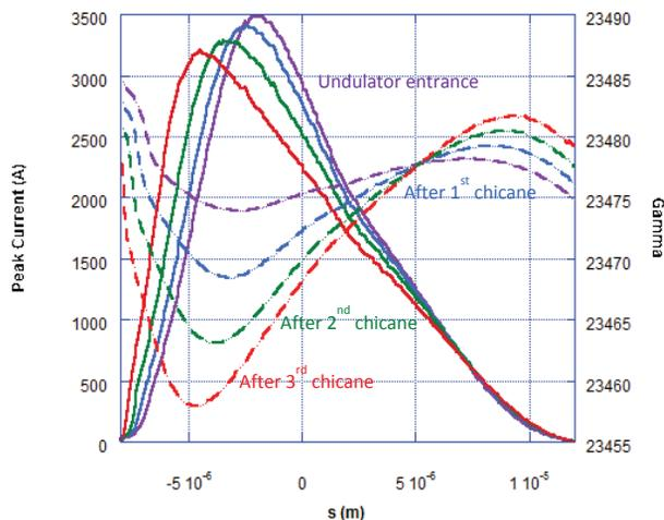
Figure 4: The CSR-induced reduction in peak current (solid lines) and slice beam gamma (dashed lines) as functions of the electron bunch position at three different undulator locations: purple = undulator entrance, blue = after the first chicane, green = after the second chicane, and red = after the third chicane.
