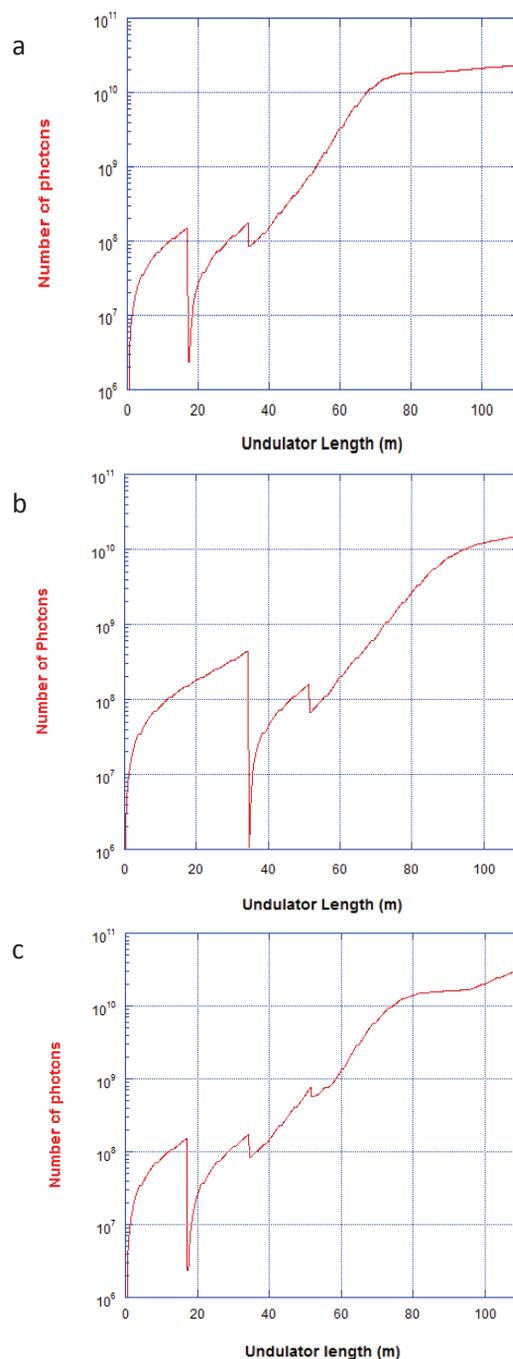
Figure 5: a) Plots of the number of photons versus undulator length for the DS configurations a) two-filter AB; b) two-filter BC; and c) three-filter ABC.
