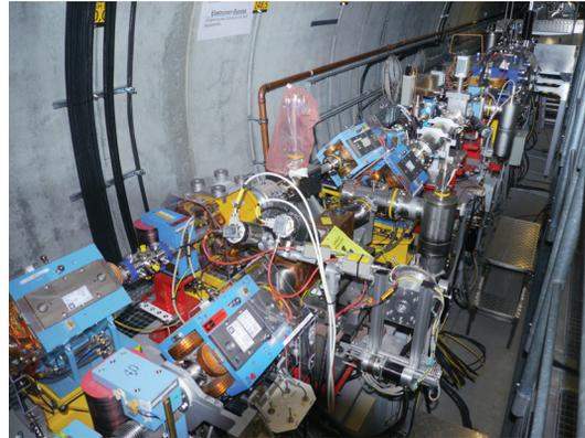
Figure 1: The first elements of the extraction arc leading the electrons to the new beamline FLASH2 are depicted on the left hand side. The beamline on the right hand side is FLASH1.
