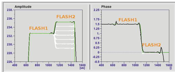
Figure 3: RF amplitude (left) and phase (right) of accelerating modules. The RF pulse length (800  $\mu$ s) is split in two parts, one for each beamline. Both, the amplitude and the phase have different settings for FLASH1 and FLASH2. The units of the horizontal axes are microseconds. The unit for the RF amplitude is energy gain in MeV and the unit for the RF phase its degree.
