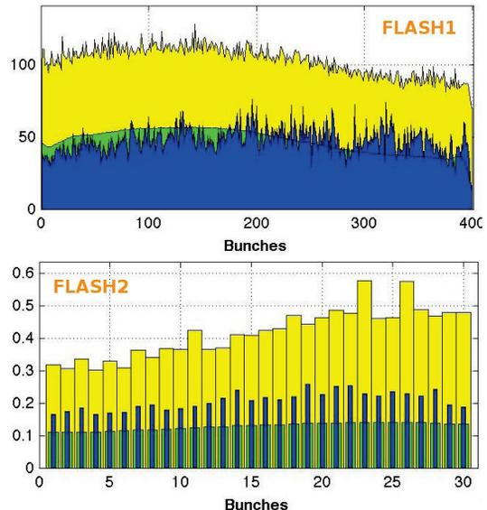
Figure 4: SASE pulse energy per bunch (in a.u.) for 400 bunches in FLASH1 (upper plot) and for 30 bunches in FLASH2 (also in a.u.). Blue: Actual value, Green: Average, Yellow: Maximum.
