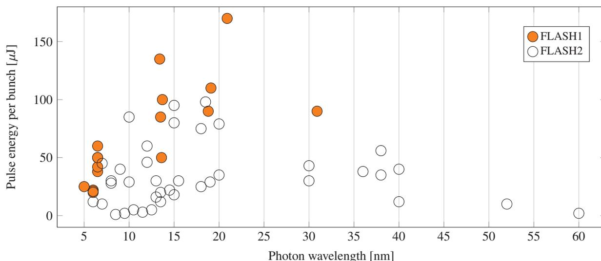
Figure 6: SASE pulse energies per bunch for photon wavelengths delivered by FLASH1 and FLASH2 achieved during parallel SASE operation in the period from June 2015 to August 2015.
