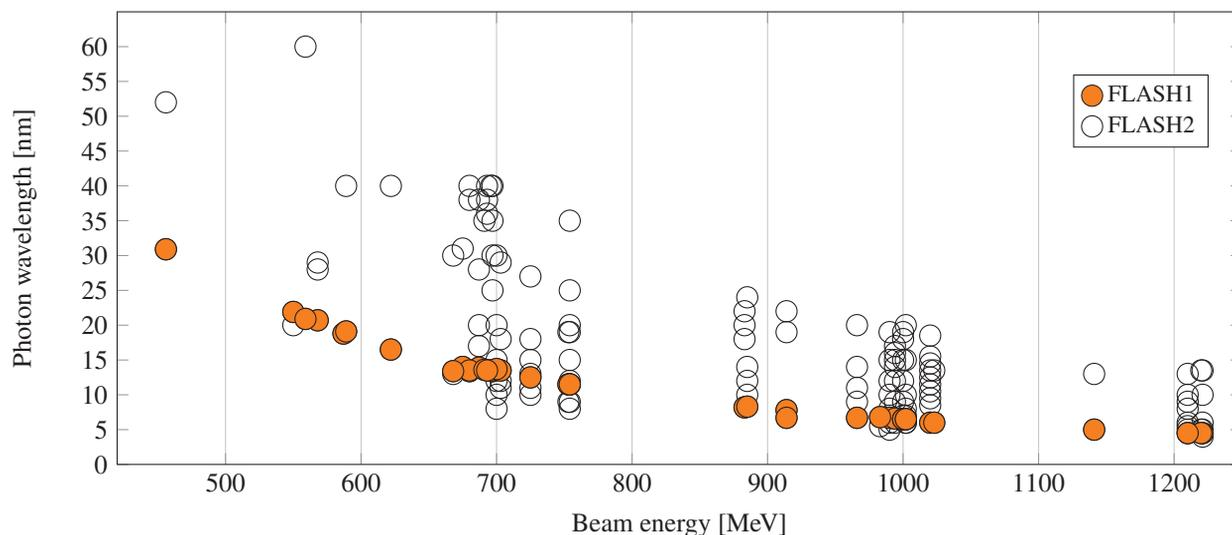
Figure 5: Photon wavelengths achieved in the FLASH1 and FLASH2 beamlines during parallel SASE operation in the period from August 2014 to August 2015. The photon wavelength in FLASH1 is determined — due to the fixed gap undulator — by the electron beam energy. FLASH2 is equipped with a variable gap undulator and the wavelength can be varied at fixed electron beam energy by changing the gap size.
