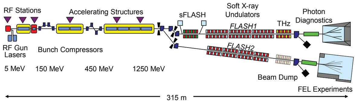
Figure 2: Schematic layout of the FLASH facility including the superconducting linac, the bunch compressors and the undulator beamlines FLASH1 and FLASH2. The location of a seeding experiment sFLASH is indicated.
