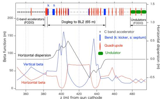
Figure 5: Beam optics and magnet configuration of the BL2 transport line.
