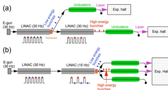
Figure 1: Multi-beamline schemes of XFEL facilities, (a) conventional layout and (b) SACLA.
