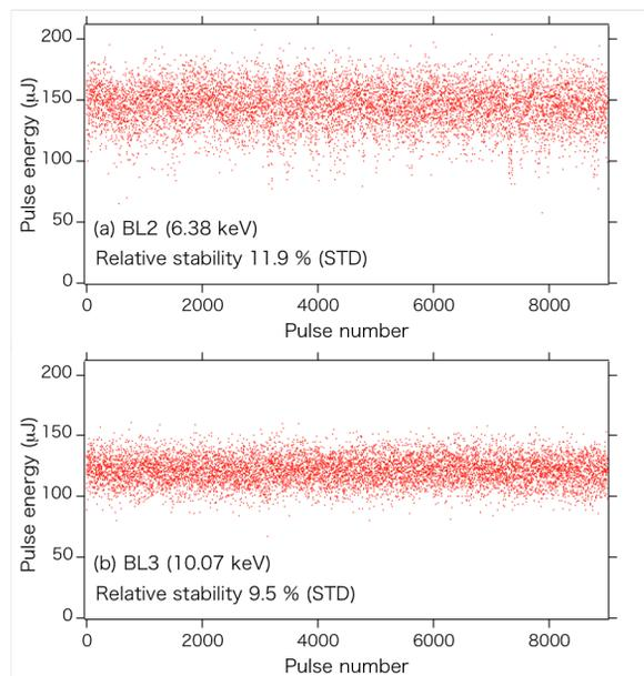
Figure 7: Stability of the photon pulse intensity, (a) BL2 and (b) BL3. Red dots are single-shot results. The electron beam energy is 7.8 GeV. The undulator K-values are 2.85 and 2.1 for BL2 and BL3 respectively.
