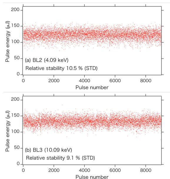
Figure 9: Stability of the photon pulse energy, (a) BL2 and (b) BL3. Red dots are single-shot results. The electron beam energy is 6.3 GeV for BL2 and 7.8 GeV for BL3. The undulator K-values are 2.85 and 2.1 for BL2 and BL3 respectively.
