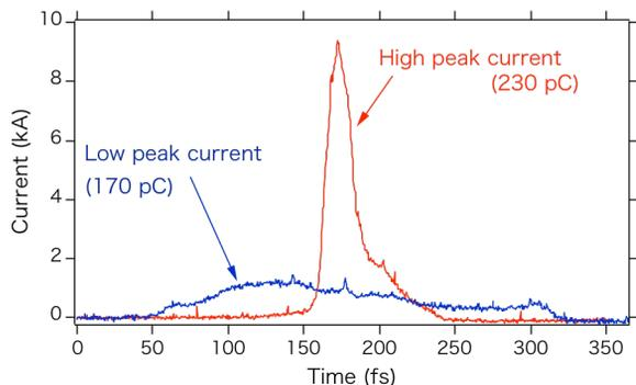
Figure 6: Longitudinal electron bunch profiles measured by a C-band RF deflector.
