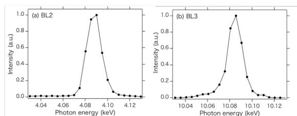
Figure 8: Averaged laser spectra measured at (a) BL2 and (b) BL3.
