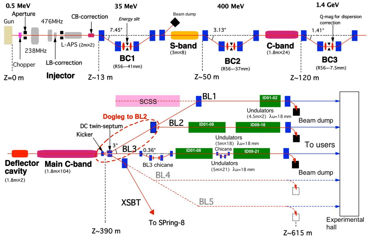
Figure 2: Schematic of SACLA facility.
