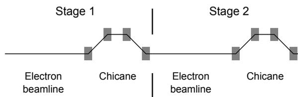
Figure 1: Schematic layout of a two-stage longitudinal space-charge amplifier (LSCA) configuration [1].
